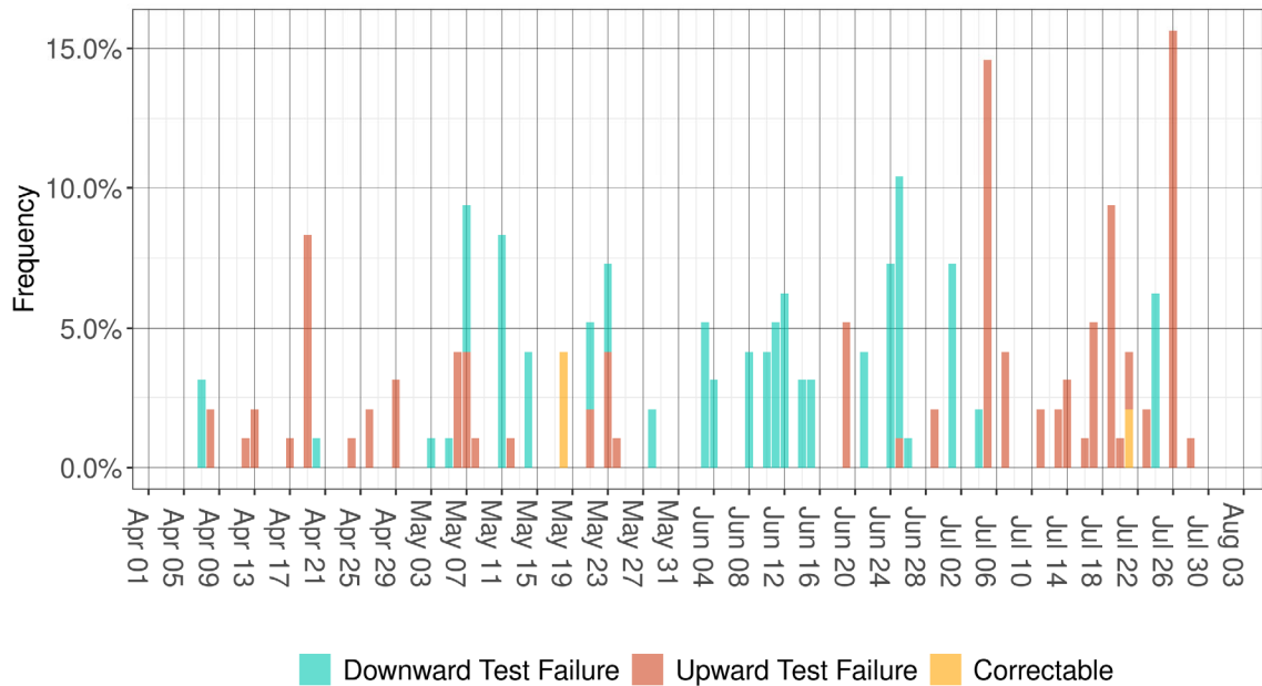
Figure 7: Frequency of Flexible Ramping Sufficiency test failures in the EPE BAA
