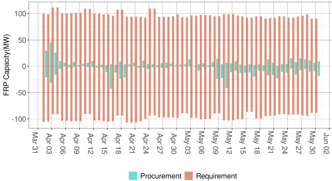
Figure 8: Daily Average requirement and procurement of upward flexible ramping in the FMM for PNM BAA
