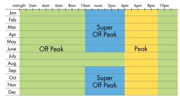
The analysis showed that throughout the year, on both weekdays and weekends, supply is expected to be constrained during the peak hours from 4 p.m. to 9 p.m. when the sun is setting and solar output is declining. During the months of July and August, the supplies are even more limited during peak hours, and higher demand begins as early as noon.
