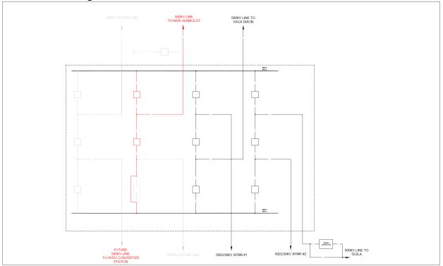
Figure I.1-3: Interconnection to Collinsville 500 kV Substations
