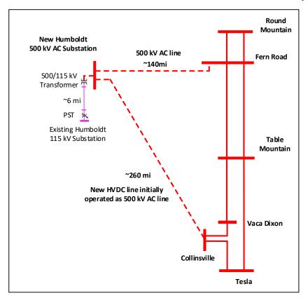
Figure I.1-1: Overall Plan to Interconnect Humboldt 500 kV to CAISO System
