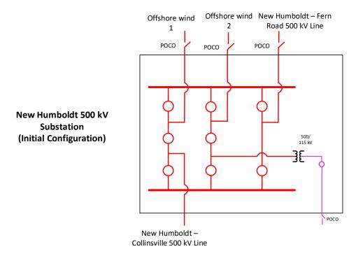
Figure I.1-2: Schematic Diagram of the Humboldt 500/115 kV Substation
