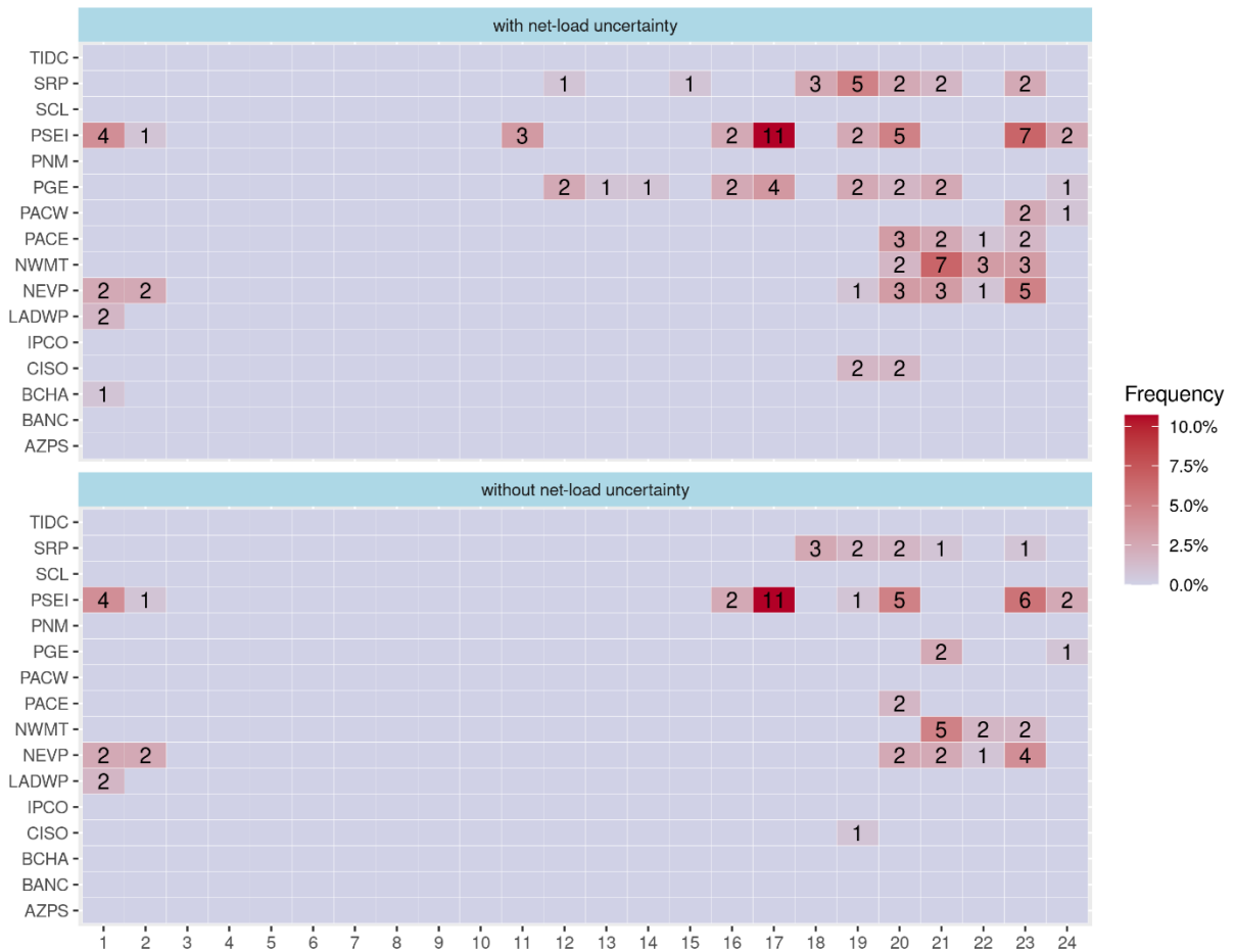
Figure 81: Daily Frequency of upward capacity test failures for all EIM BAAs under two scenarios
