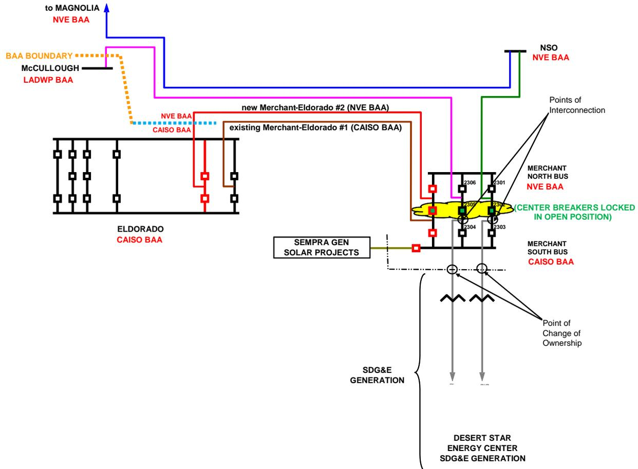
The configuration in Figure 1 will result in, south bus of Merchant Switchyard, and the Merchant-EI Dorado #1 circuit being included within the CAISO BAA. The tie breakers in the 230 kV Merchant Switchyard will remain locked in open position and isolated during this interim phase and will serve as the demarcation boundary between the NVE BAA (North Bus and its associated connections) and CAISO BAA (South Bus and its associated connections).
