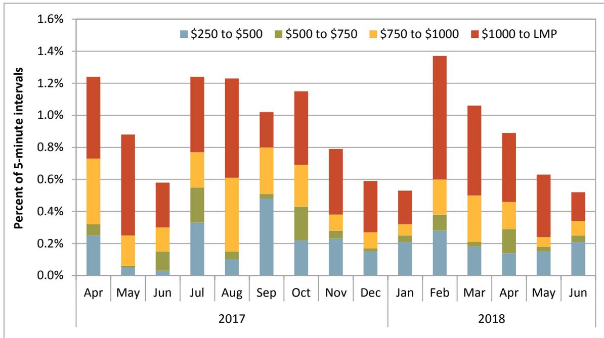
**Figure 1.8 Frequency of under-supply power balance constraint infeasibilities (5-minute market)**
