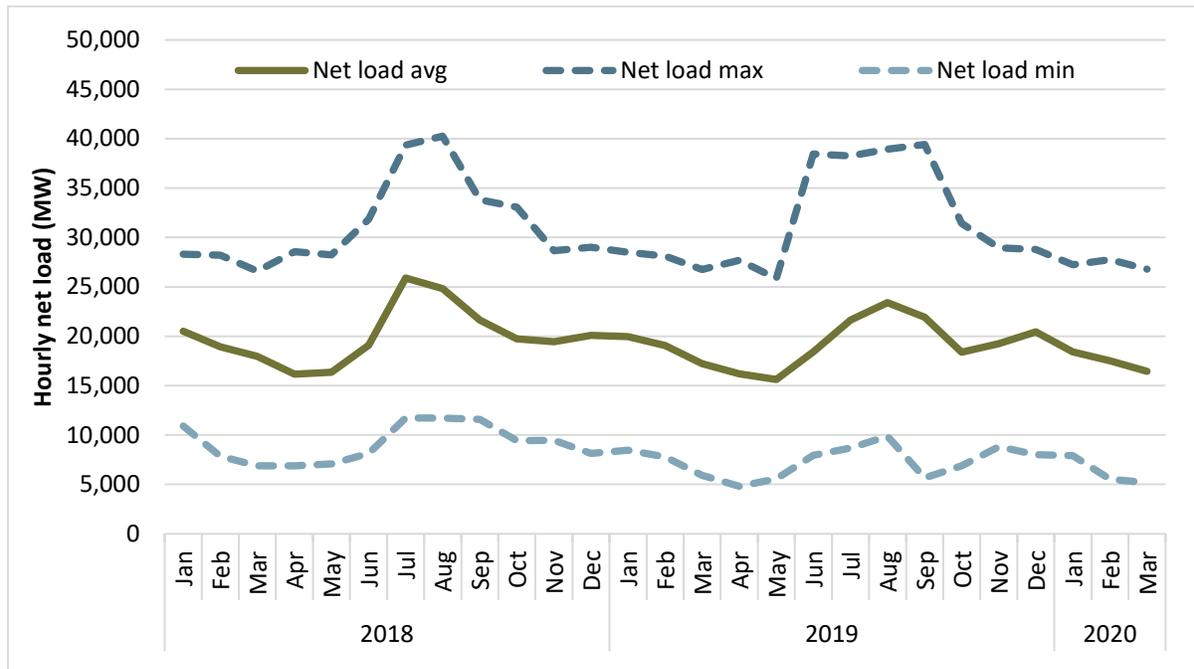
Figure 1.11 offers insight into how behind-the-meter solar resources affect ISO load. Generation from utility scale wind and solar resources indirectly affects load by influencing how other generation sources must meet demand after wind and solar have been factored out, i.e., the net load. Conversely, generation from behind-the-meter solar resources directly reduces the amount of load that must be met by generation from the ISO market, regardless of source.
