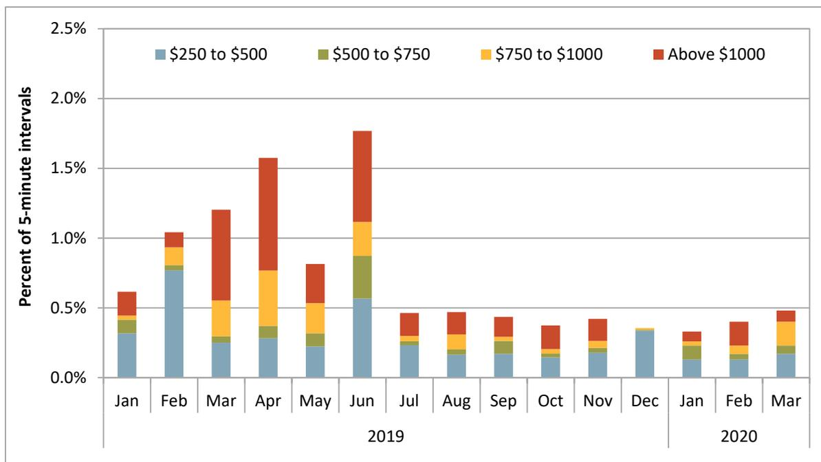
**Figure 1.17 Frequency of under-supply power balance constraint infeasibilities (5-minute market)**
