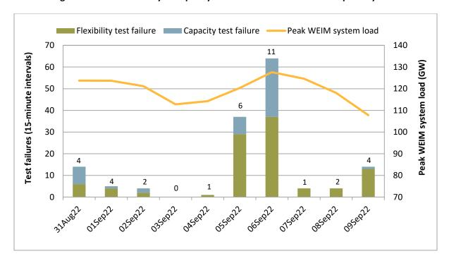
Figure 2.1 Flexibility or capacity test failures across WEIM footprint by date
