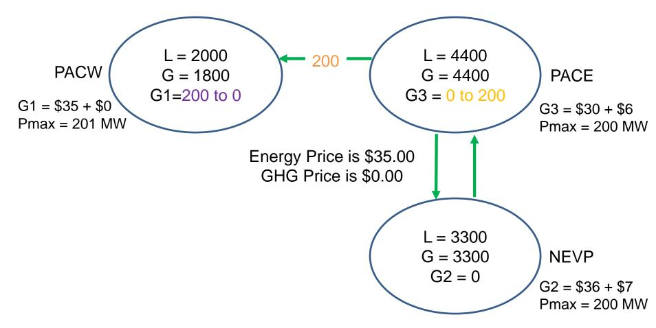
G3 increases its output and G1 reduces its output because G3 is lower cost than G1. LMP outside ISO is \$35
