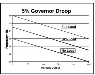
4. **Governor limits.** Turbine control systems that provide adjustable limits to governor valve movement (valve position limit or equivalent) should not restrict travel more than necessary to coordinate boiler and turbine response characteristics. *Graph showing relation between general*
