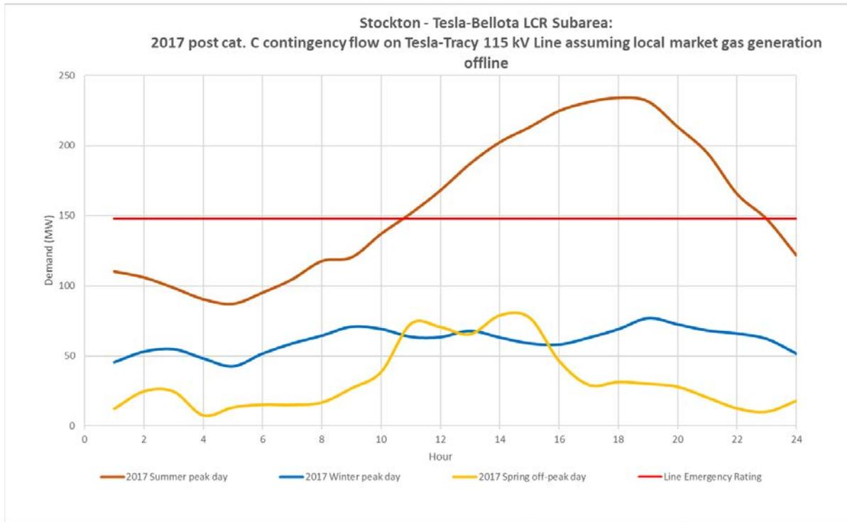
Figure 3.5-28 Tesla-Bellota LCR Sub-area 2017 Limiting Post Contingency Hourly Profiles
