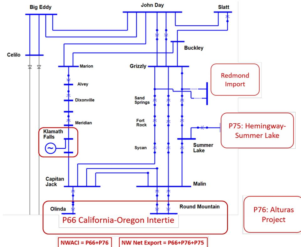
BPA performed a detailed study to quantify the correlation between the parameters impacting the NW Net Export capability. Figure 4.2-3 shows that a total of 5,100 MW on COI and Path 76 is achievable under a wide range of Path 75 flows when Klamath Falls generation is dispatched at high levels, which based on historical data is expected to be the case in summer months.
