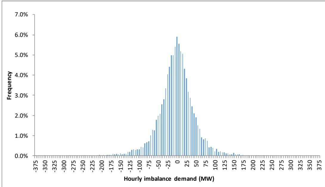
**Figure 2. Hourly imbalance energy demand compared to total load for the TEP BAA
