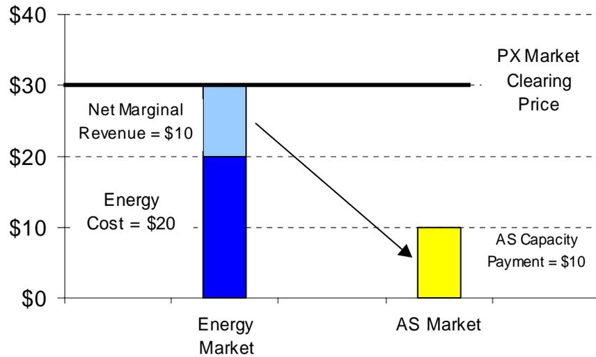
**Figure 6-9. Illustrative Example of the Cost of Providing A/S**
