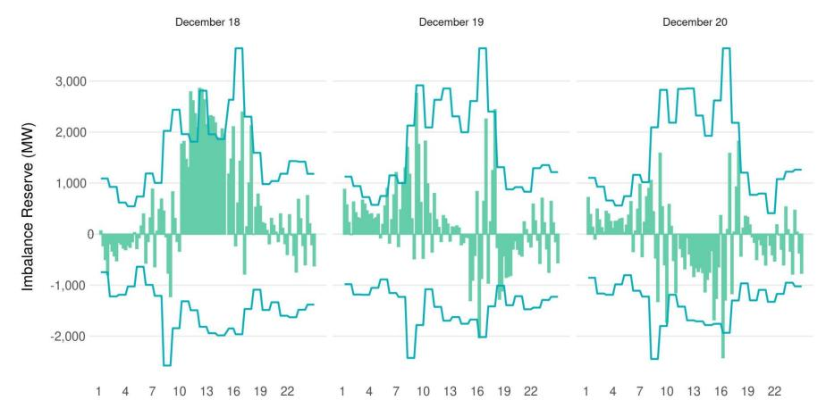
Green bars stand for actual imbalances while blue lines represent the upward and downward IR requirements
