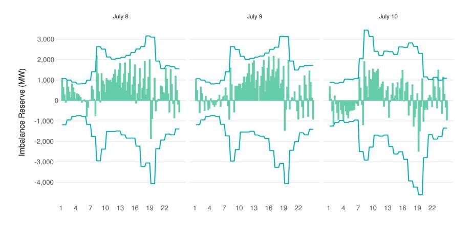
Green bars stand for actual imbalances while blue lines represent the upward and downward IR requirements
