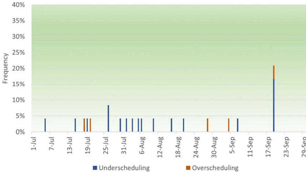
Figure 57: Frequency of Balancing Test Failures for the PGE BAA
