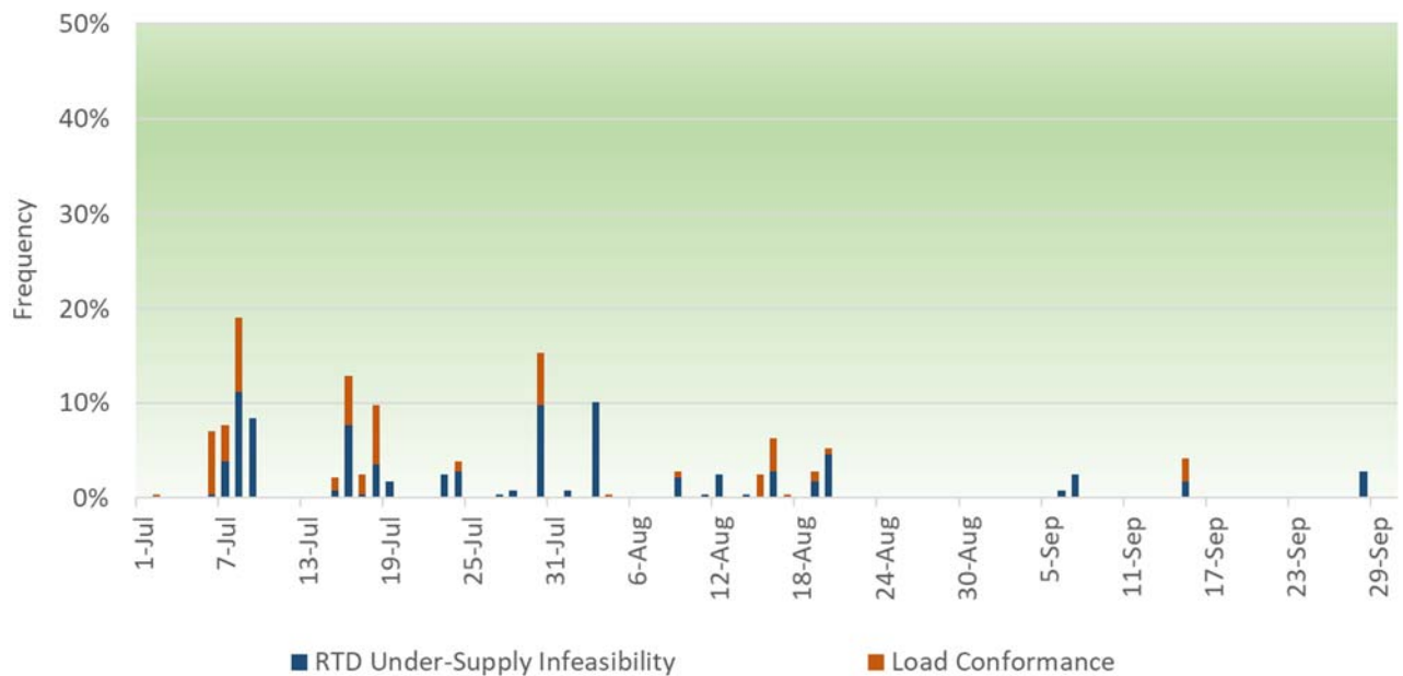
Figure 42: Frequency of RTD Power Balance infeasibilities in the NV Energy BAA
