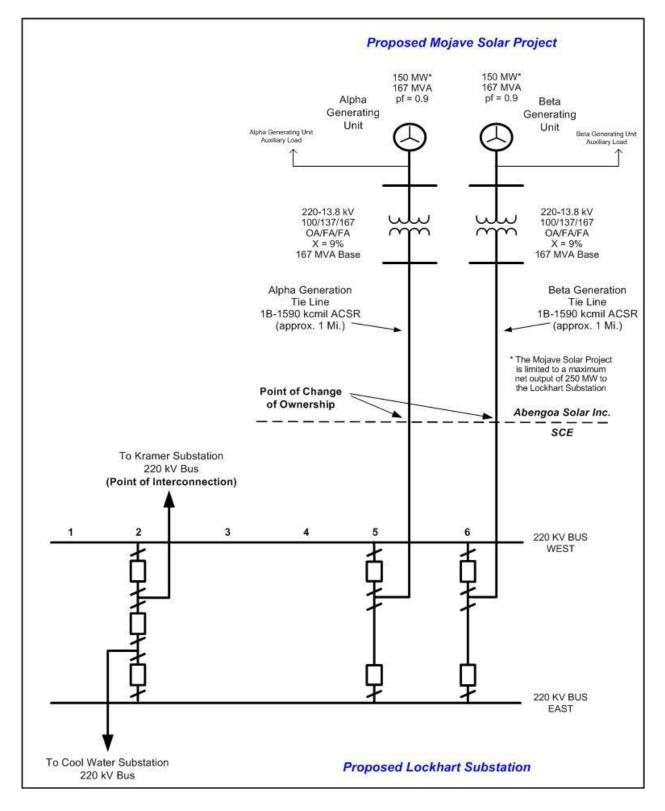
6. One-Line Diagram of Interconnection to Lockhart Substation
