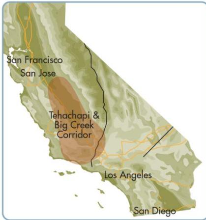
WECC Path 26 — three 500 kV transmission lines between PG&E's Midway substation and SCE's Vincent substation with Whirlwind 500 kV loop-in to the third line;
