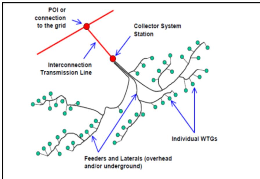
Figure 6.2-4: Equivalent model of a wind farm or solar PV plant for use in power flow and dynamic stability studies.
