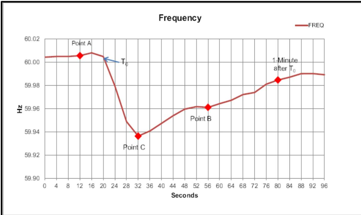
The system frequency performance is acceptable when the frequency nadir post-contingency is above the set point for the first block of the under-frequency load shedding relays, which is set at 59.5 Hz.
