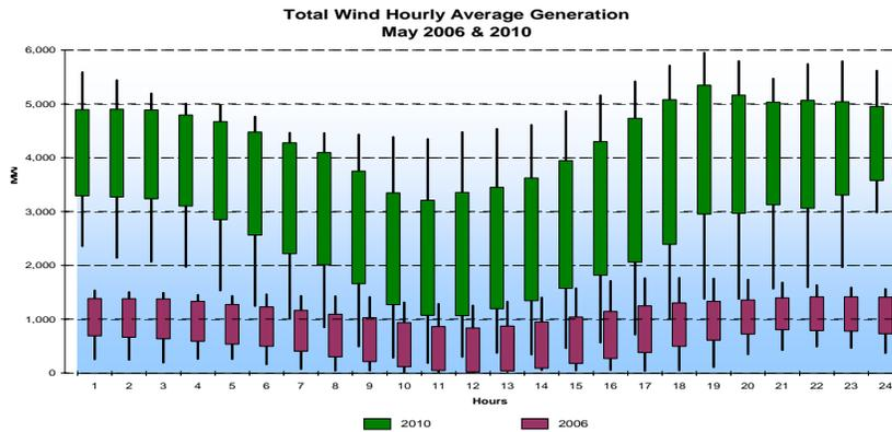
Figure 3: Actual 2006 Hourly Wind Generation vs. Expected 2010 Hourly Wind Generation
