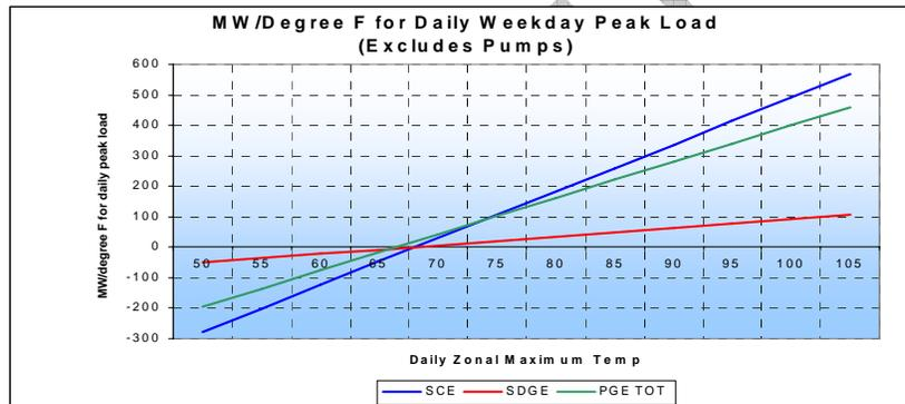
Figure 1: Temperature vs. Peak Load Variation
