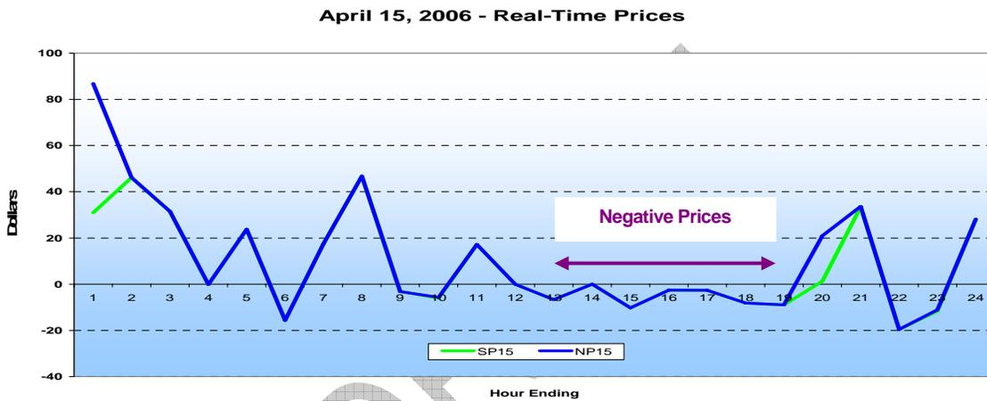
Figure 27: Real Time Prices During Overgeneration Conditions
