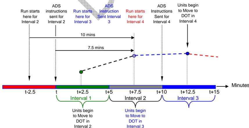
Figure 16: MRTU Timeline for five-Minute Dispatch
