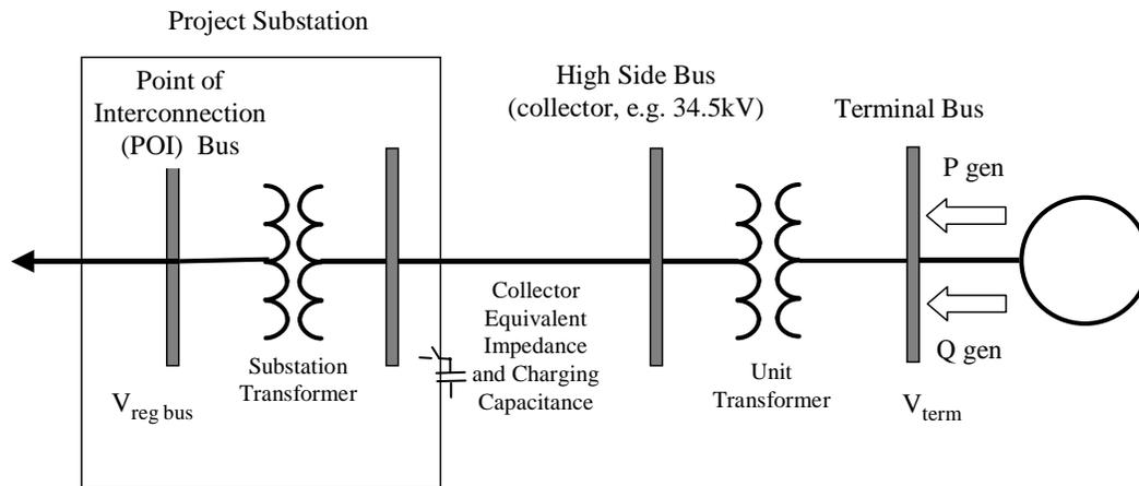
Figure 1: Wind Plant Equivalent Model
