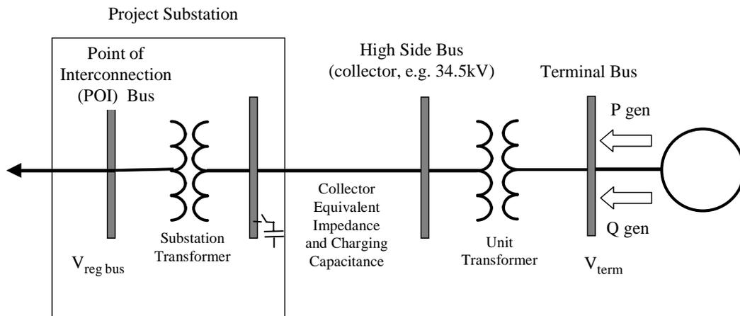
Figure 1: Wind Plant Equivalent Model.
