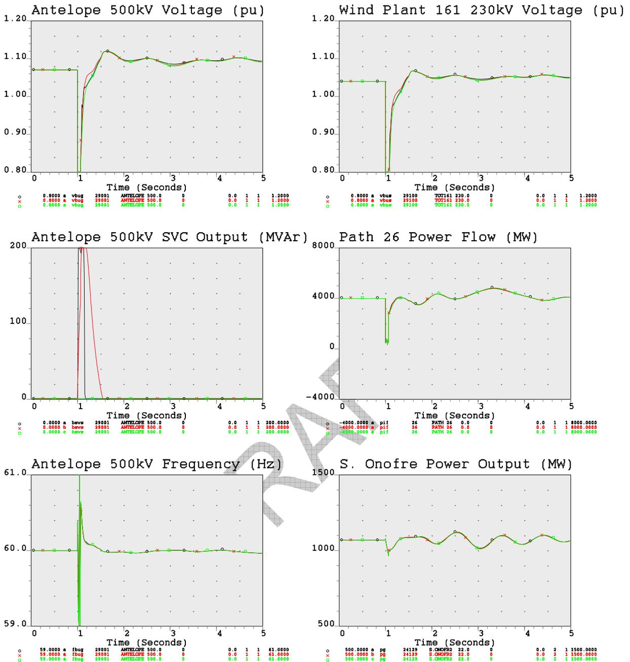
Figure 5. System Performance Overview, Vincent-Antelope 500 kV Double Line Outage, 2010 Heavy Summer Load, Full Wind Plant Output, Mixed Technology (Black=Nominal SVCs, Red=Modified SVCs, Green=No SVCs).
