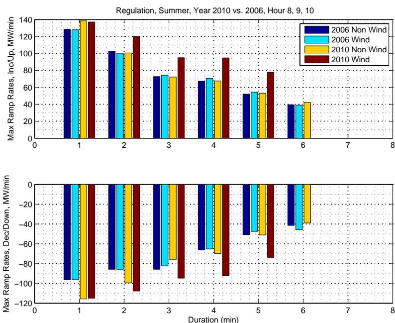
Figure 24: Regulation Ramp Duration
