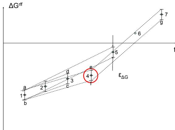
Figure 8: "Swinging Door" Algorithm - Idea
