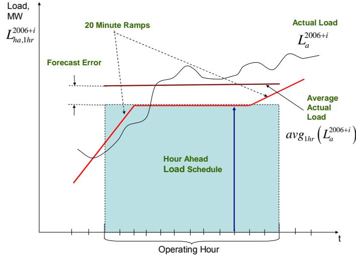
Figure 4: CAISO Simulated Hour Ahead Load Schedule (Red Line)
