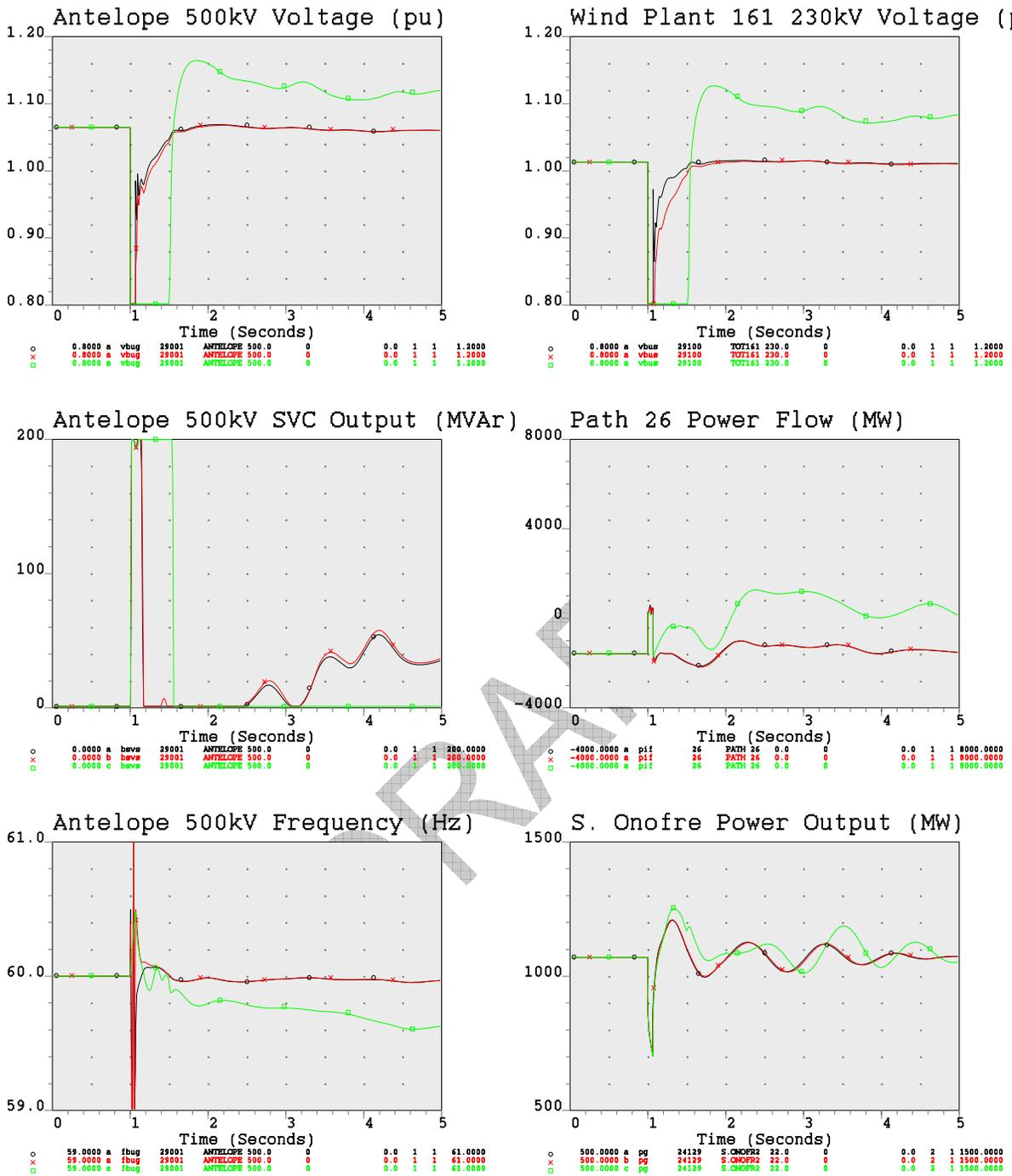
Figure 4: System Performance Overview, Vincent-Antelope 500 kV Double Line Outage, 2012 Light Spring Load, Full Wind Plant Output, (Black=100% Type 3 Doubly Fed, Red=Mixed Technology, Green=100% Type 1 Induction Generator).
