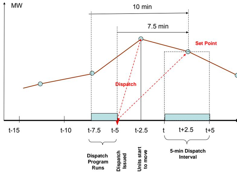
Figure 3: CAISO Real Time Dispatch Timeline
