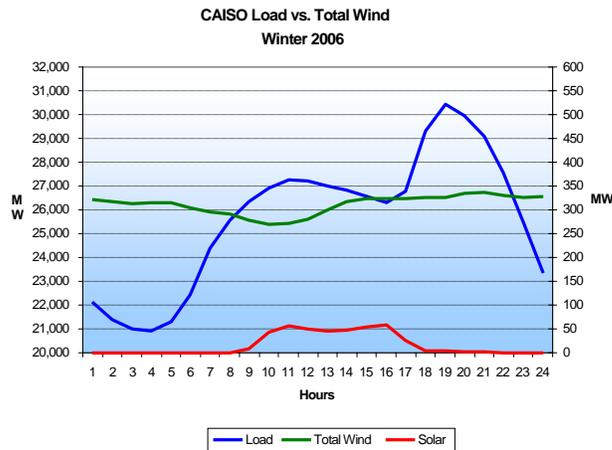
Figure 11: Actual System Load, Wind Generation and Solar Generation for Winter 2006
