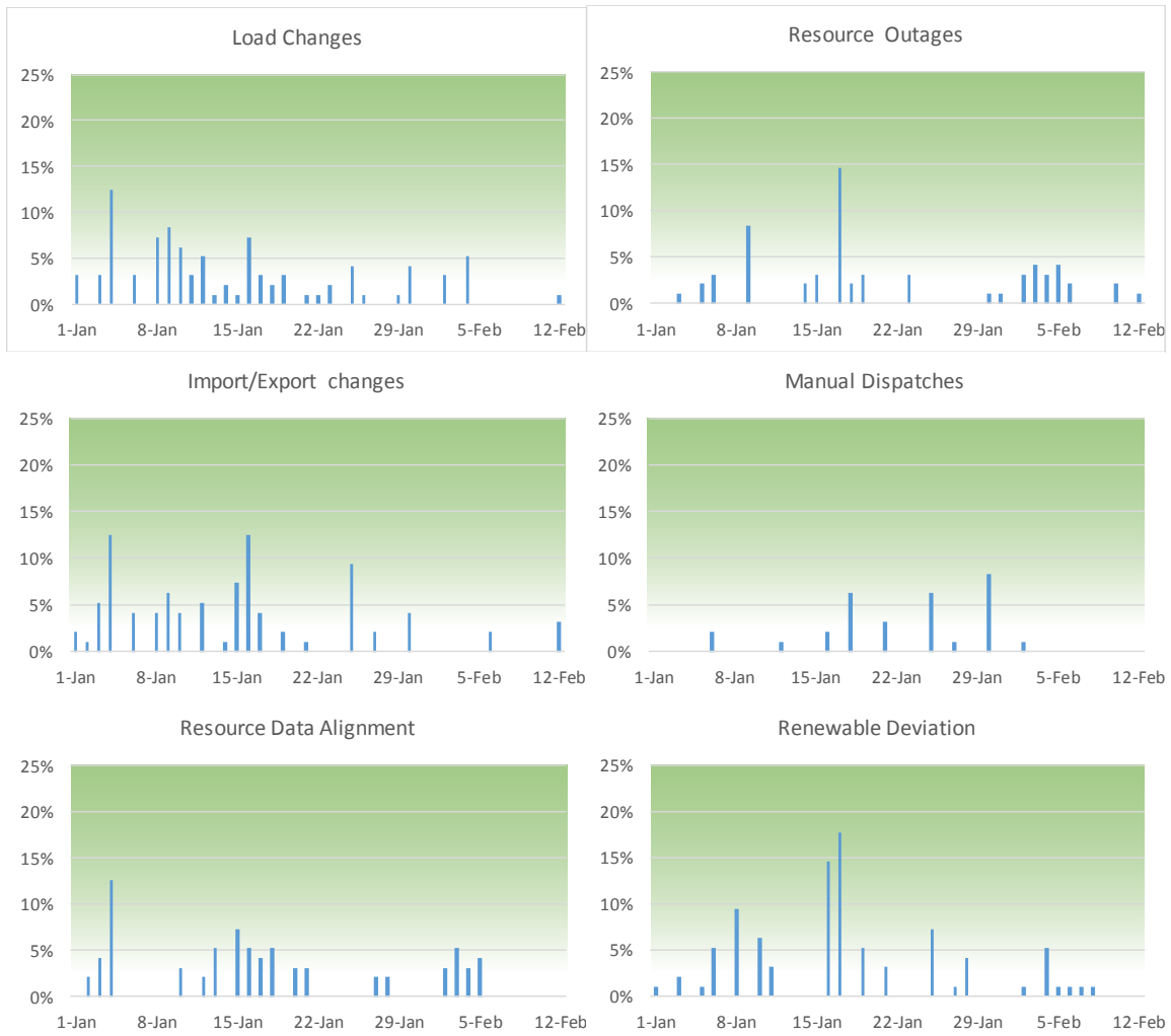
Figure 13: Frequency of reasons leading to power balance infeasibilities in the fifteen-minute market. Both PAC West and PAC East combined.
