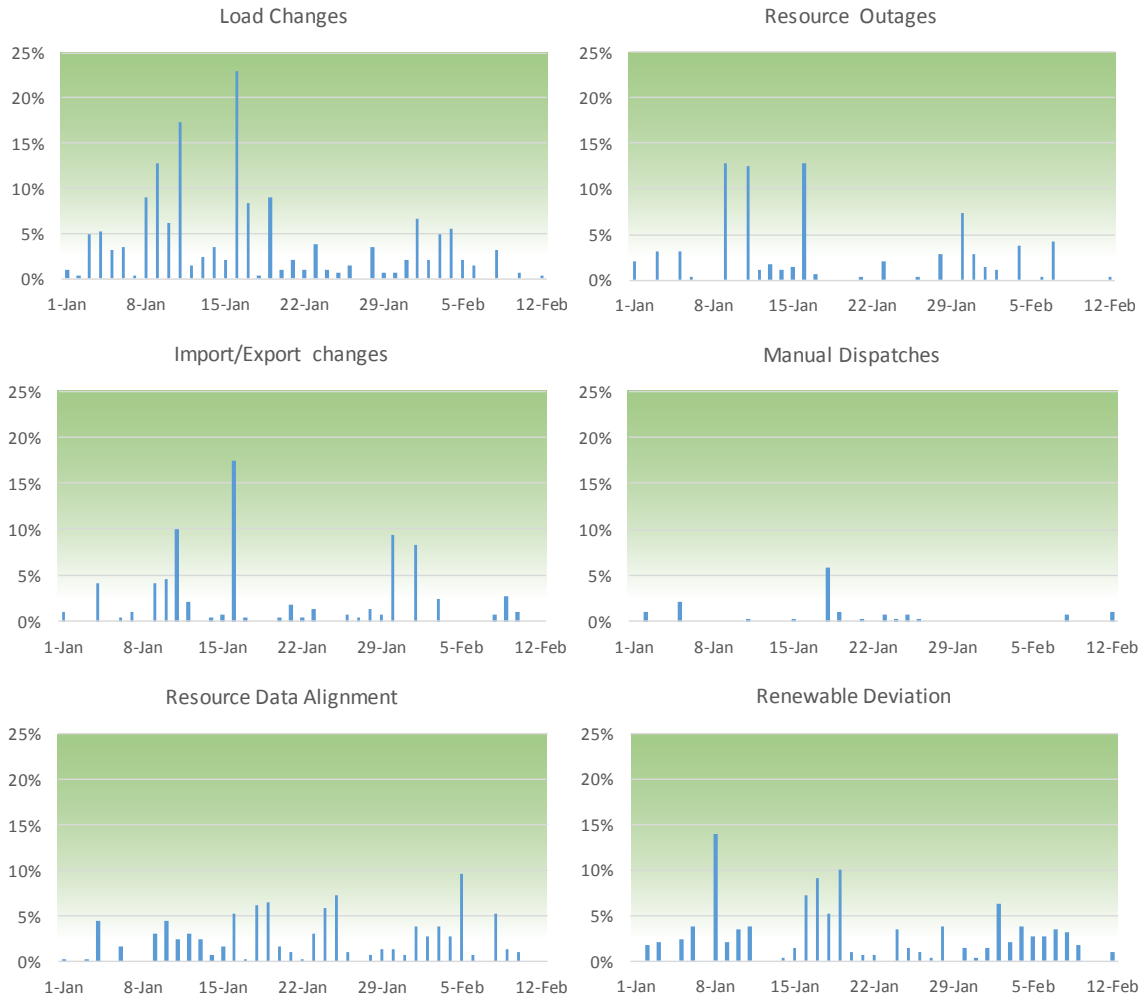
Figure 14: Frequency of reasons leading to power balance infeasibilities in the five-minute market. Both PAC West and PAC East combined.
