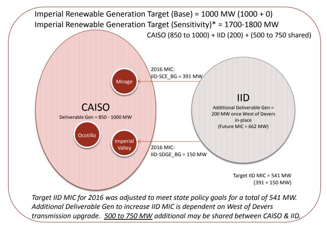
CAISO's explanation of its last 3 years of deliverability assessments highlights that the methodology does not align deliverability allocation between CAISO and IID interconnections based on the actual physical constraints of the two interconnected systems.
