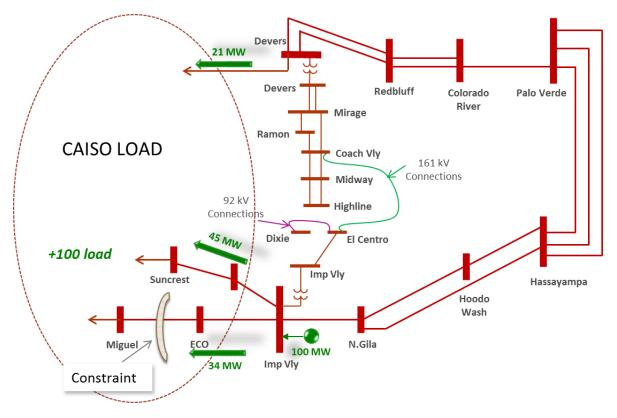
Figure 6. Impact of 100 MW Generator Interconnected at Imperial Valley Substation on ECO-Miguel 500 kV Constraint
