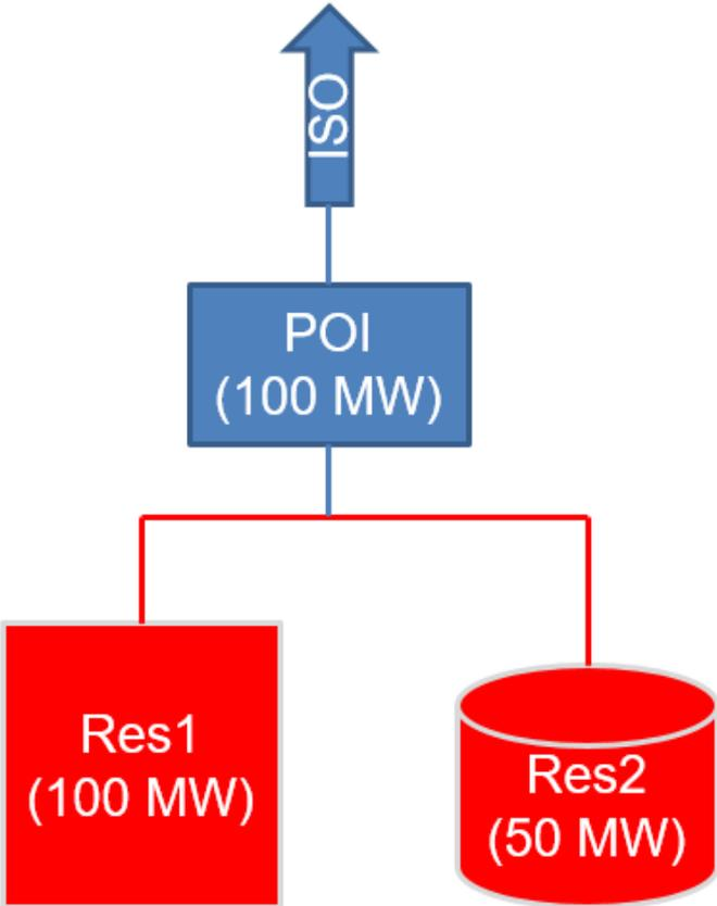
In this example, Resource 1 and Resource 2 are co-located with each other. Further, because the aggregate value of the maximum generation from these two resources exceeds the limit at the point of interconnection, the ISO will require application of the aggregate capability constraint to prevent the combined dispatch from these resources from ever exceeding the 100 MW interconnection limit.
