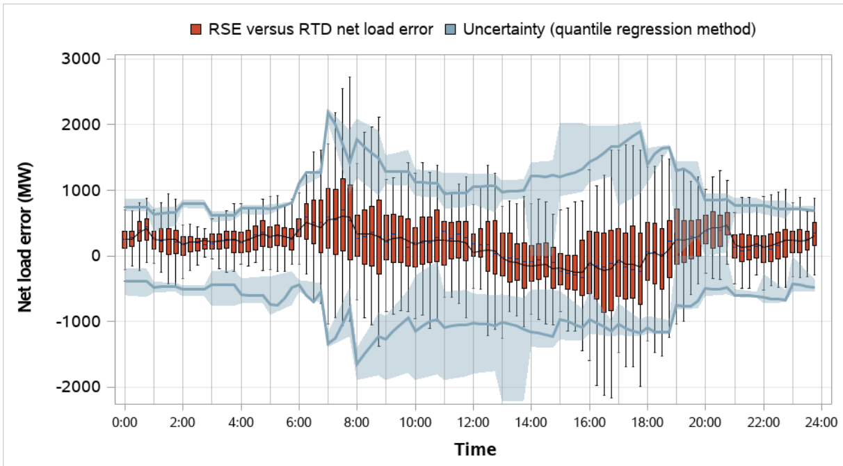
Figure 4.5 CAISO distribution of RSE and RTD net load error and comparison to RSE uncertainty (weekdays, June 2023)
