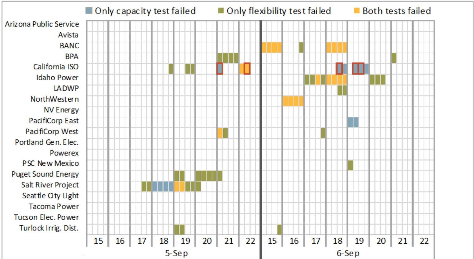
**Red boxes indicate intervals when CAISO should have failed capacity test if available battery capacity was correctly calculated.**
