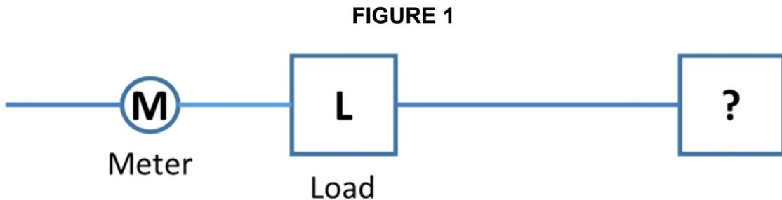
The load may be a pure load, or it may be offset by behind-the-meter generation or other devices, such as battery storage. With such a meter configuration—one that lacks separate metering of behind-the-meter generation—there is no way to separate the load from the generation or vice versa. The CAISO cannot distinguish the cause of demand response behind the meter.
