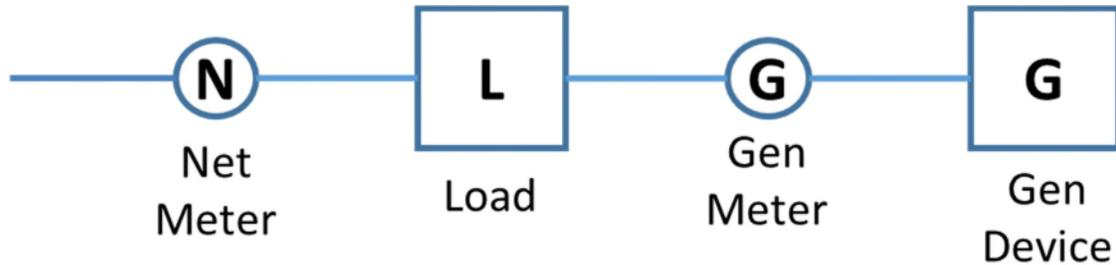
Under this configuration, the overall demand response at the location can be separated into a pure demand response (from the facility) and behind-the-meter generation energy production.
