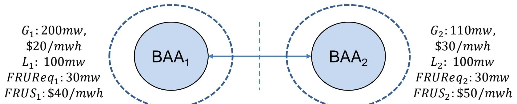
Assumption: fail sufficiency test,  $FRUReq = 30\text{mw}$  for each BAA
