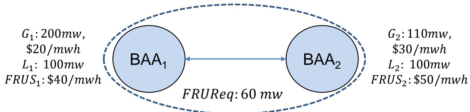
Assumption: both pass sufficiency test,  $FRUReq = 60\text{mw}$  for the group
