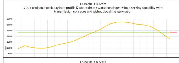
2021 projected peak day load profile & approximate worst contingency load serving capabilities with transmission upgrades; Estimated amount of storage that can be added from charging restriction perspective = 4300 MW and 43000 MWh
