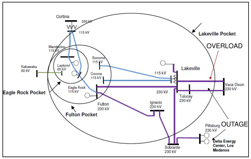
No overload in 2019 due to the line reconductoring.
