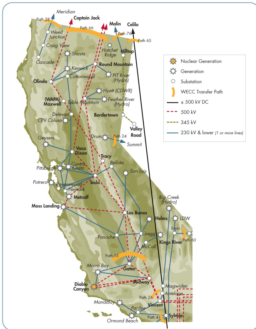
Figure 2.4-1: Map of PG&E bulk transmission system
