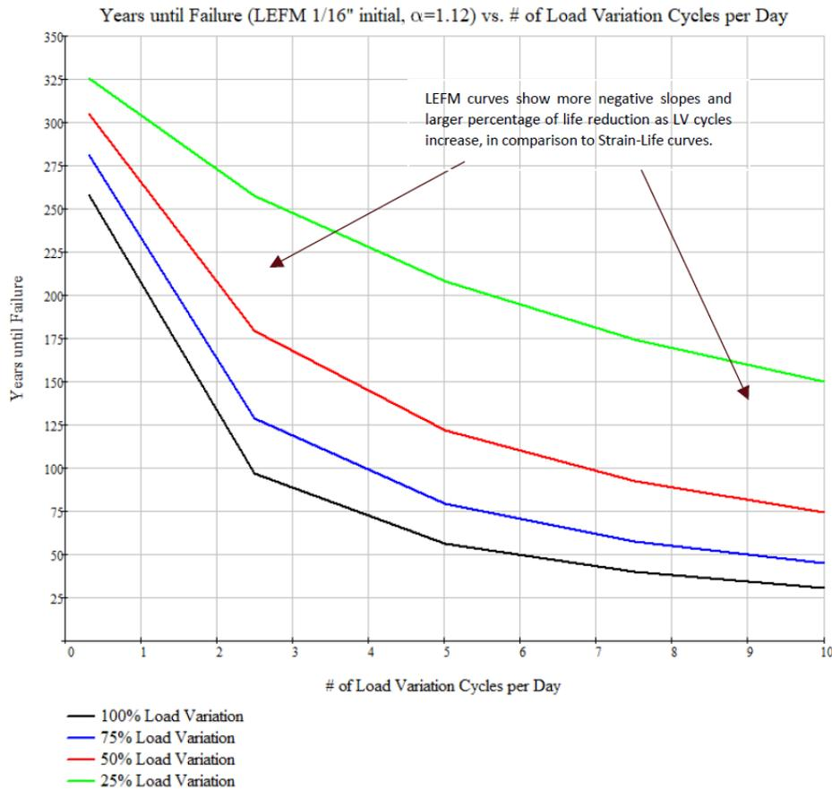
Figure 23. Infinite edge crack LEFM plot showing sensitivity to LV cycle increase.
