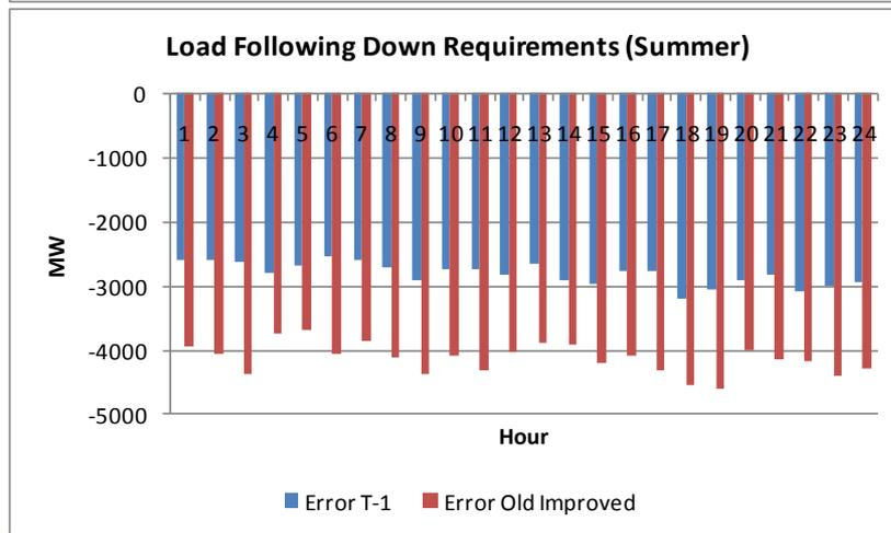
Comparison of regulation requirements using new and previous forecast error. Higher regulation requirement reflects 2010 actual T-7.5 forecast error high then 2006 assumption.
