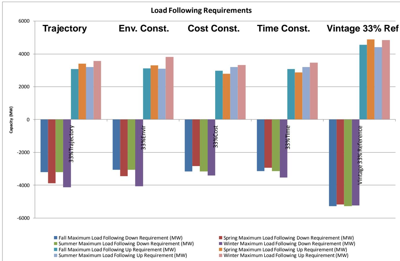
Comparison of load following requirements using refined and previous forecast error. Decrease in load following requirements reflect decrease in T-1 hour forecast errors.
