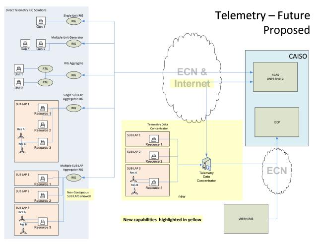
**Figure<sup>4</sup> 2- 2 Telemetry Architectural Overview**
