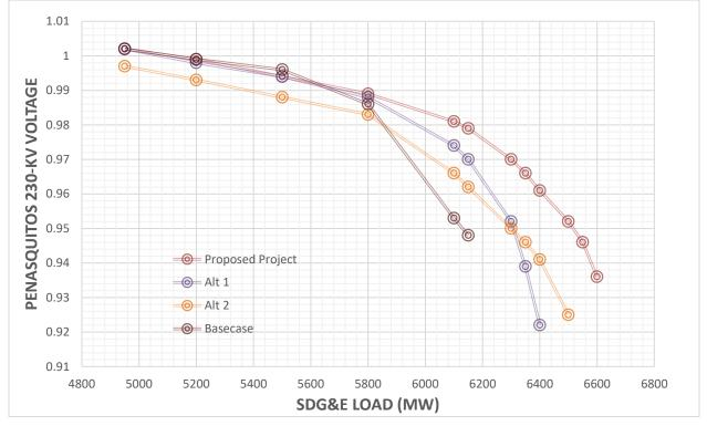
Alt 1: 230-kV line from Alberhill to Sycamore Canyon Alt 2: 500-kV line from Devers to Suncrest
