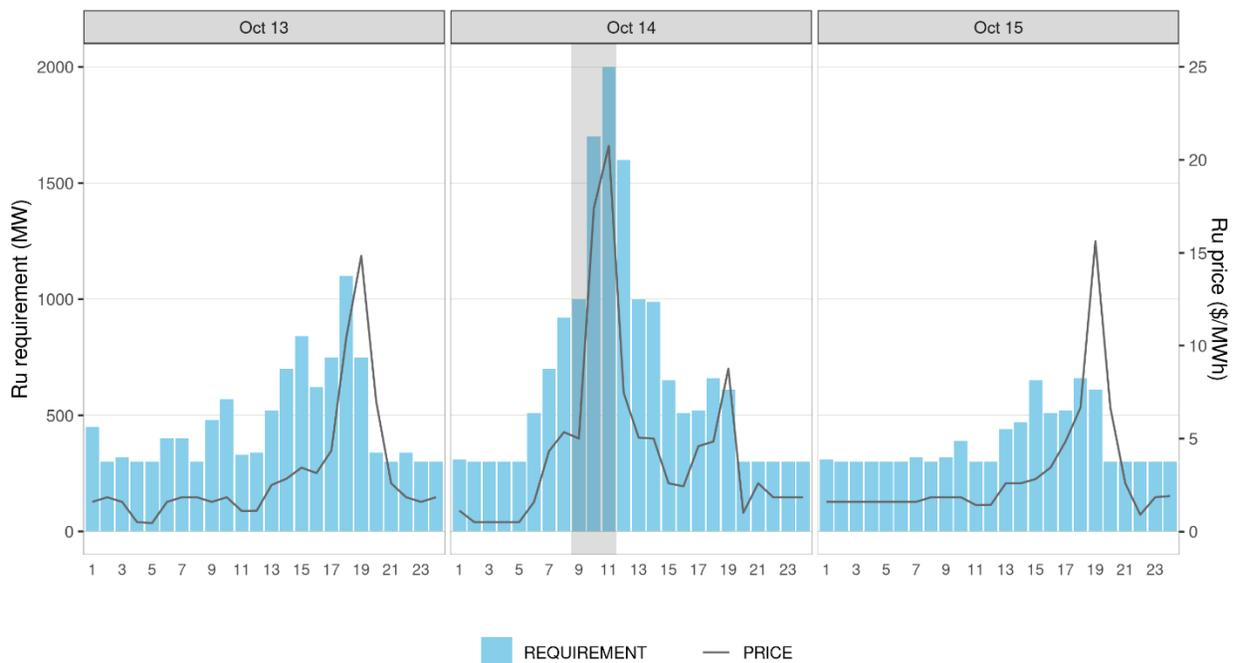
Figure 28 presents the CAISO regulation down requirement and prices in the day-ahead market. Regulation down requirements and prices from hour ending 8 through 12 are noticeably higher than a typical day.
