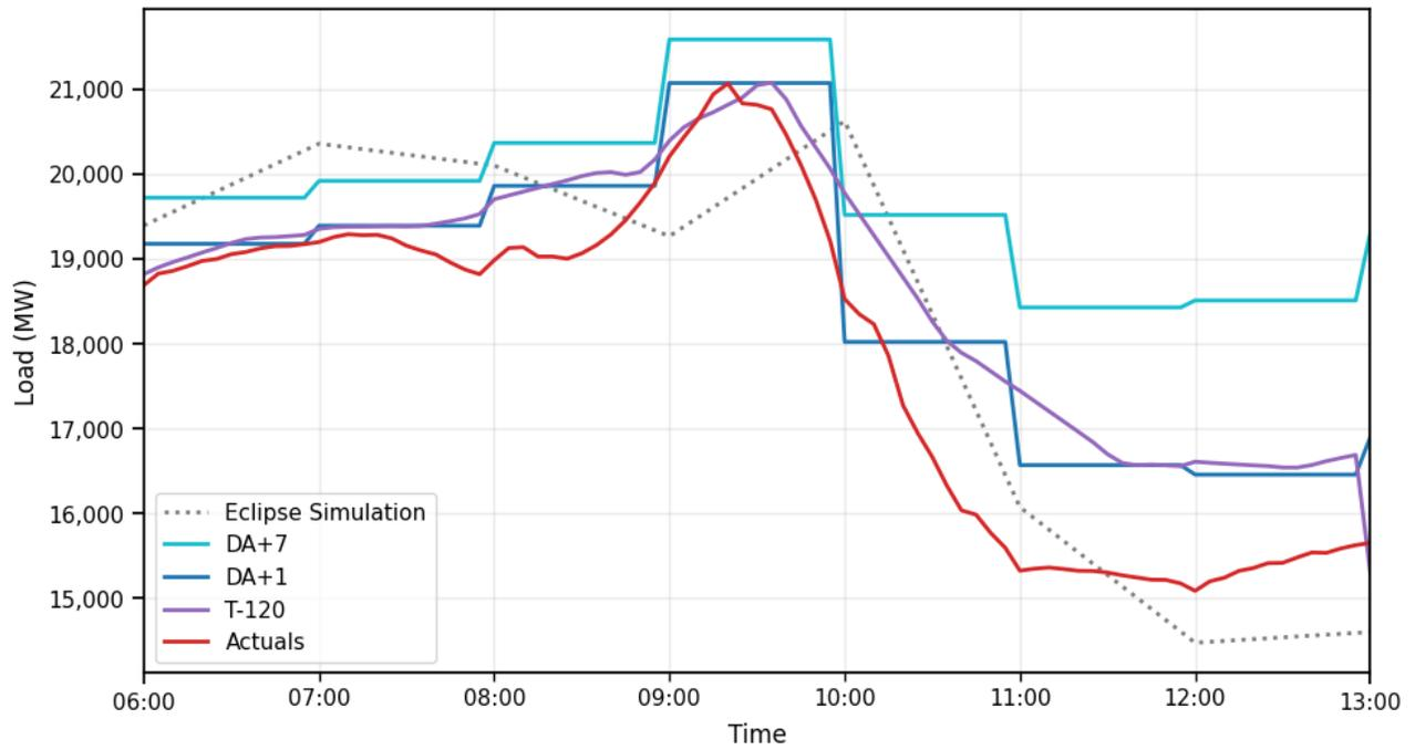
Figure 8 CAISO HASP through RTD load forecasts and actuals during eclipse timeframe
