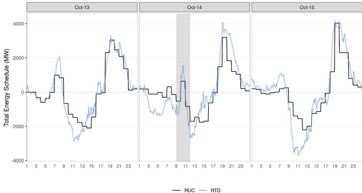
Figure 43 illustrates the energy awards for storage with prices in the RTD. The storage resources charged continuously through the morning peak hours, in anticipation of the eclipse event. During the eclipse hours, the storage resources discharged as prices reached the local peak, and charged in the midday hours after the event, when the real-time prices had turned negative.
