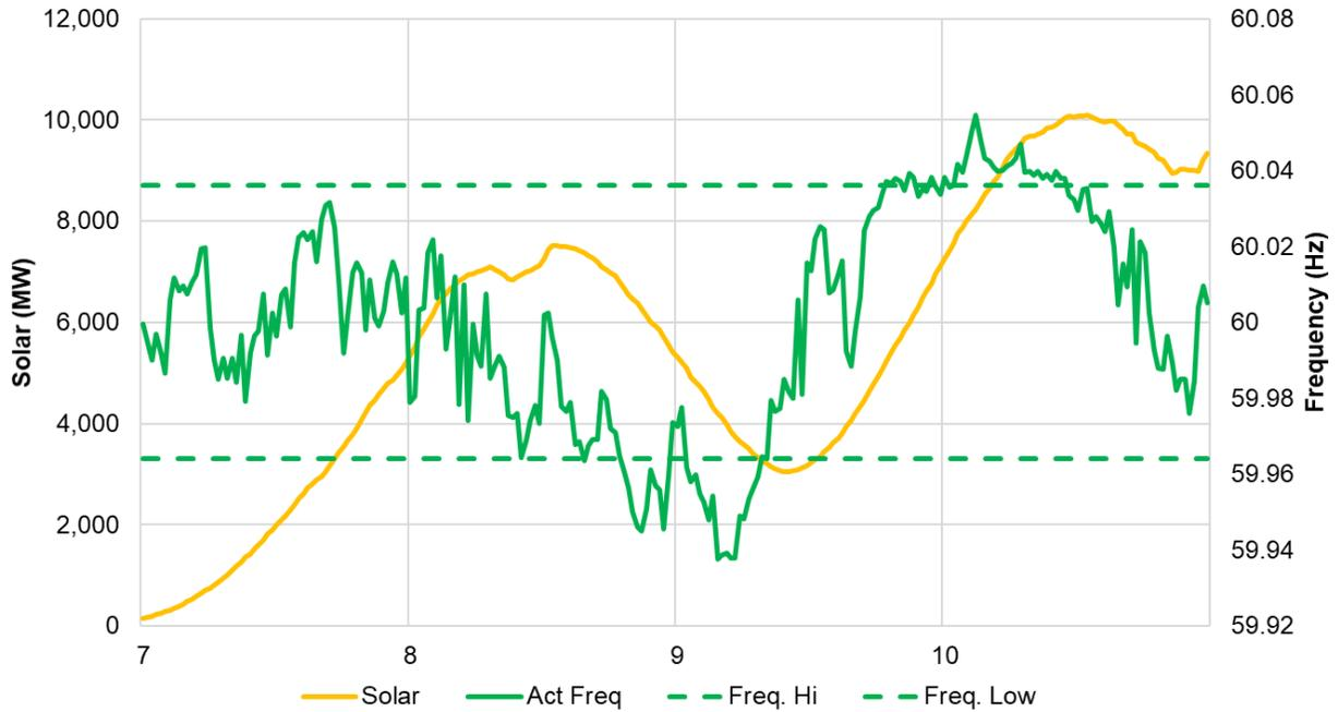
Figure 63: Solar Production vs. ACE
