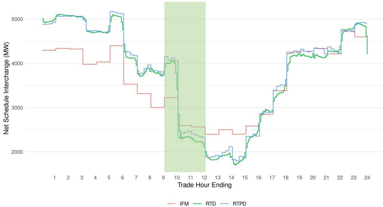
Figure 55 shows NSI on October 14 for RTD by major intertie point. The approximate time period of the eclipse is shown in light green. While there is no single intertie that drove the pattern of increased NSI during the time of the eclipse, PWVEST and MALIN500 were larger contributors.
