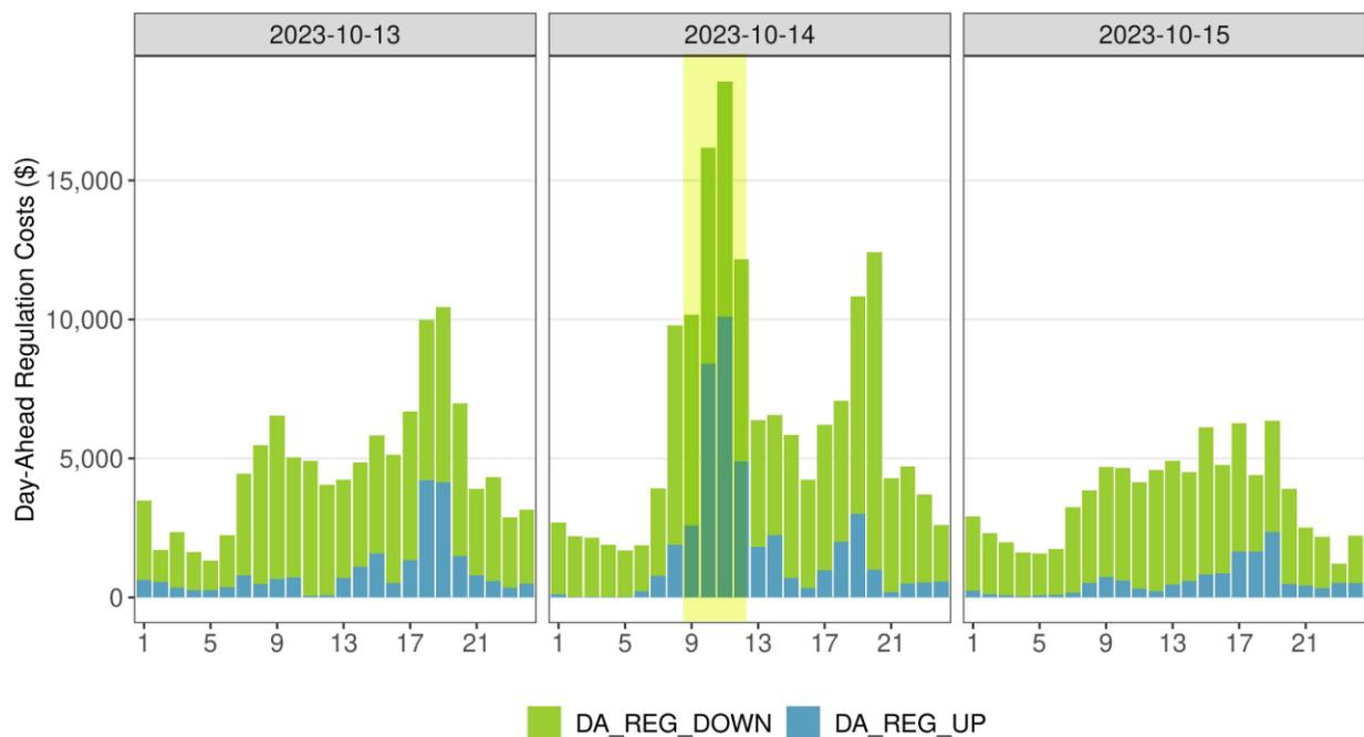
Figure 33 to 35 show a longer-term trend of regulation costs over a two-month span from September 1, 2023 through October 31, 2023. The day of the eclipse event is highlighted. The longer trend shows that regulation costs on the day of the eclipse event, October 14, were somewhat higher when compared to the surrounding days in both markets.
