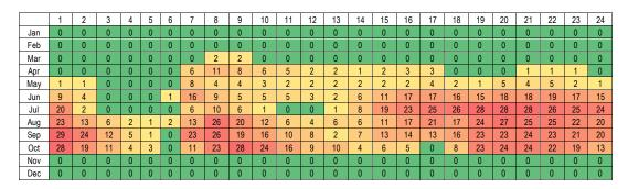
In the Alternative 3 case with the reconductoring the 115 kV lines between Oro Loma and Wilson PG&E 115 kV buses, the 115 kV congestion can be mitigated, but the 70 kV congestion under the N-1 contingency of the Panoche-Mendota 115 kV line still remained.
