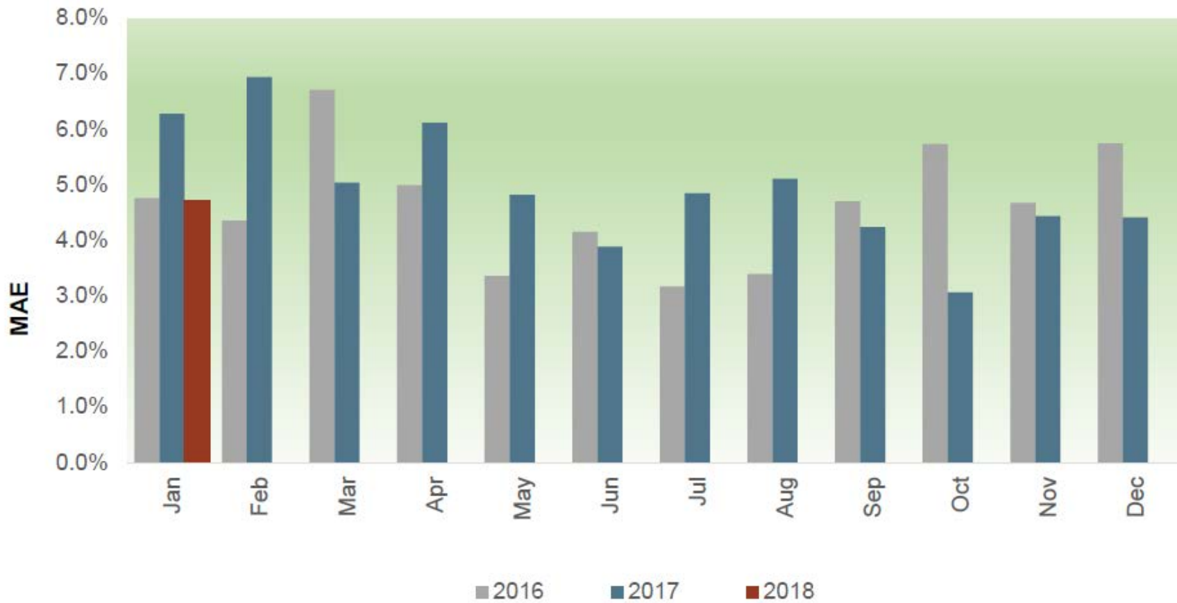
Day-ahead solar forecast accuracy. Mean Average Errors (MAE) by month. Source: Market Performance and Planning Forum. February 20, 2018 – Slide #74.
