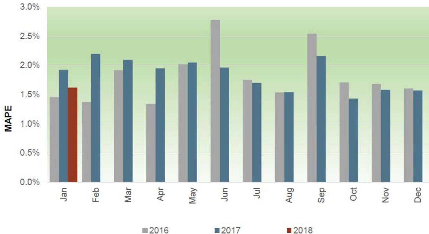
Day-ahead load forecast accuracy. Mean Absolute Percent Error (MAPE) by month. Source: Market Performance and Planning Forum. February 20, 2018 – Slide #71.
