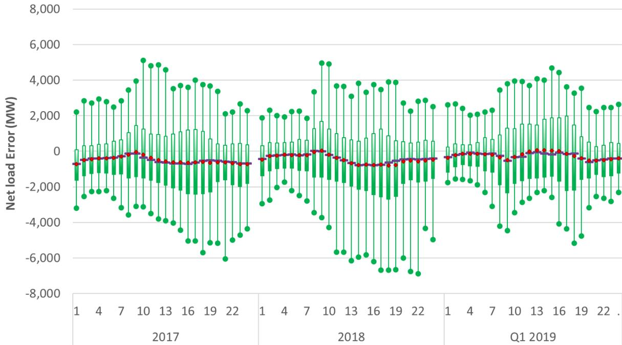
In general, the net load errors between markets is smaller when no operator adjustments are considered for the load (*i.e.* load conformance and RUC net short). These metrics also deduct any infeasibilities caused by operator adjustments because these infeasibilities do not lead to more supply being dispatched.
