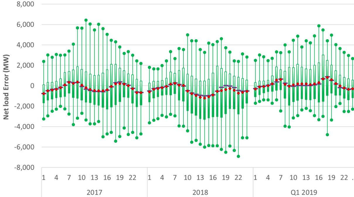
Figure 49: Hourly profile of net load differences between RUC and RTD
