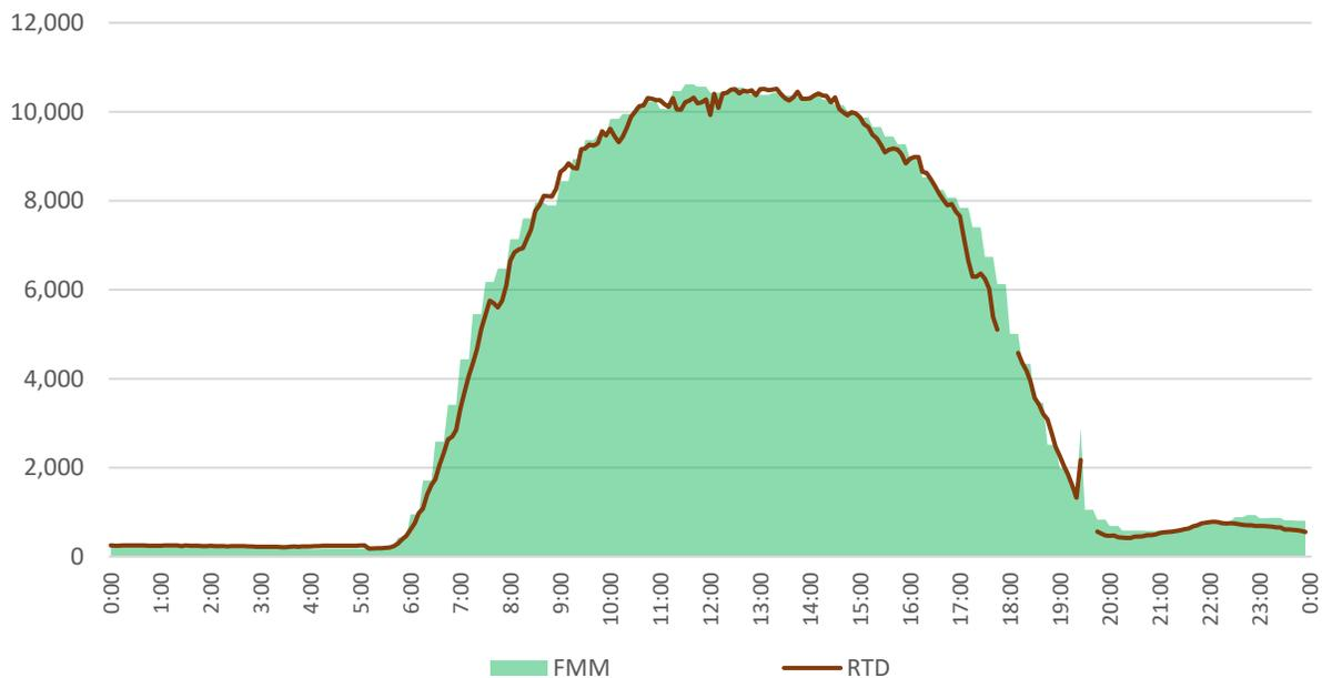
There was a sharp decline in VER generation around 5:00 PM: VER output dropped from 7,657 MW at 5:00 PM to 6,295 MW at 5:15 PM, resulting in a loss of 1,362 MW within fifteen minutes. The total RTD VER output was 1,106 MW below the FMM awards.
