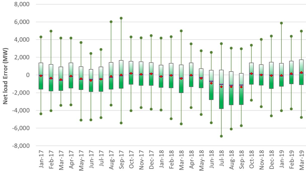
Figure 53: Monthly profile of net load differences between RUC and RTD
