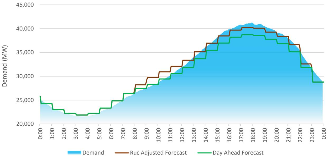
One challenge to grid operators was that the real-time load came in about 2,500 MW above the day-ahead load forecast<sup>31</sup>. There was a RUC adjustment made to increase the demand that RUC used to clear during its run, but it was still below the real-time demand. This instance represents the challenge that
