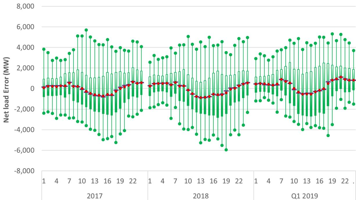
Effectively, the disregard of virtual supply shows larger net load errors in the upward direction and smaller errors in the downward direction. This is more pronounced during the midday hours, which follow an inverse profile to solar dispatch.
