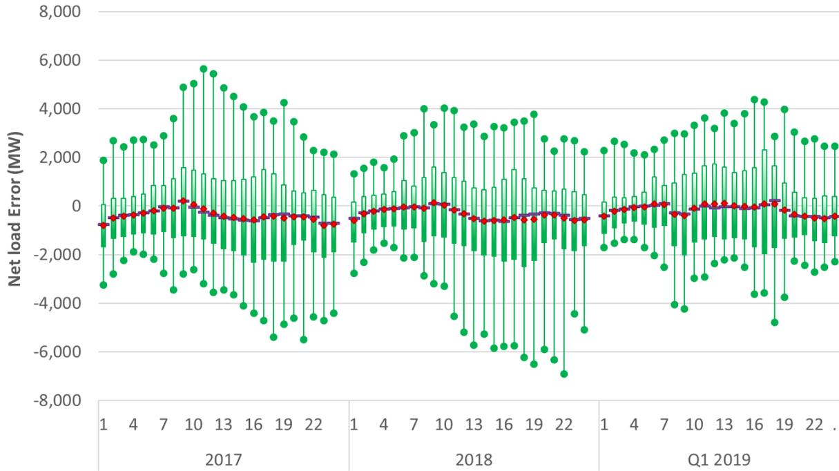
Figure 60: Hourly profile of net load differences between RUC and RTD with no load conformance
