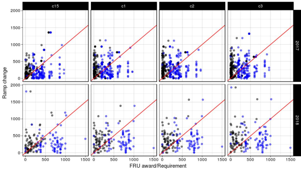
Figure 106 shows resources' ramp change and FRU award by their fuel types. Due to the multiple time intervals involved in FRU deployment in FMM, color coding is used to represent the resources' fuel types instead of matrix in Figure 91 for the RTD market. It can be seen that water and gas were dispatched the most in both 2017 and 2018, and resources that have high ramp change but were awarded little FRU are mostly gas types.
