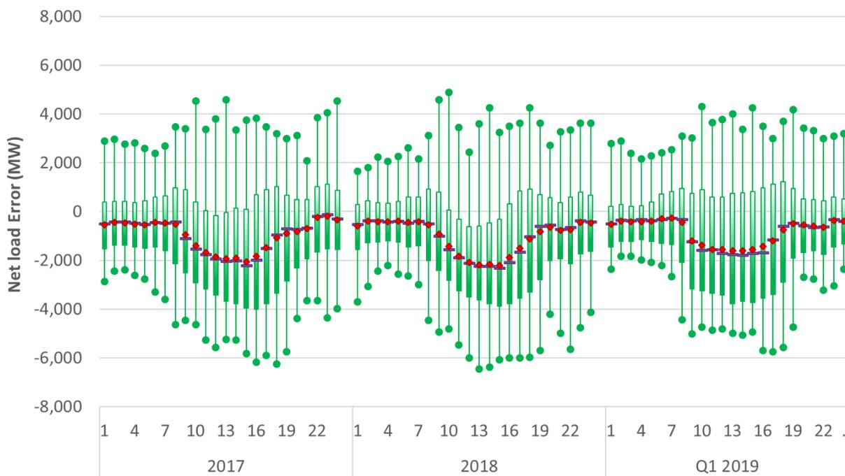
Figure 48: Hourly profile of net load differences between RUC and FMM
