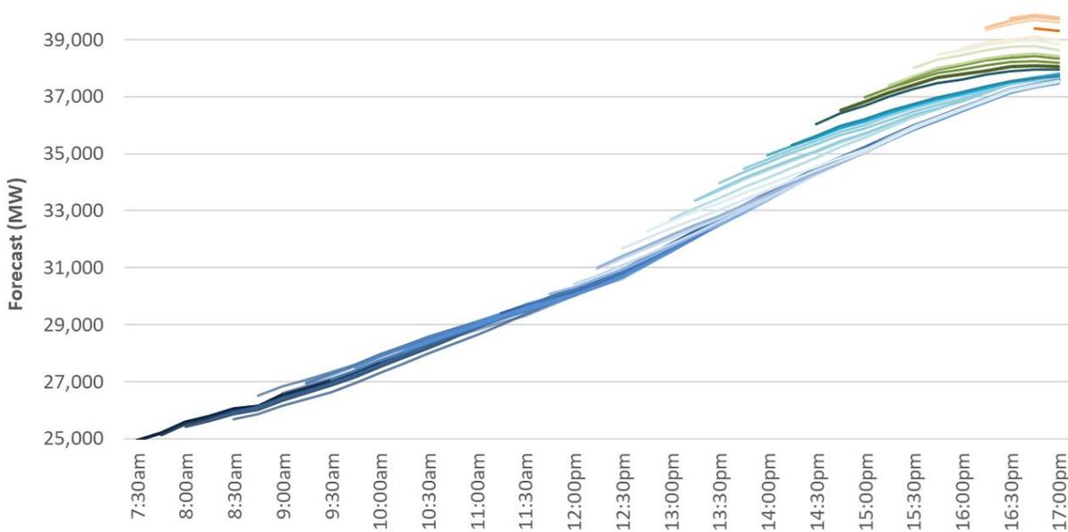
Figure 144: Evolution of load forecast at 5:00 PM on June 10
