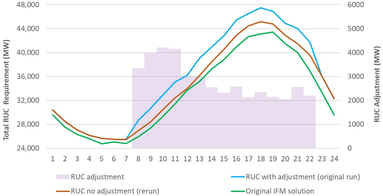
The additional requirement imposed by the adjustment increases the need for additional capacity to be cleared in RUC. Figure 136 shows the additional capacity cleared by having the additional RUC requirement.
