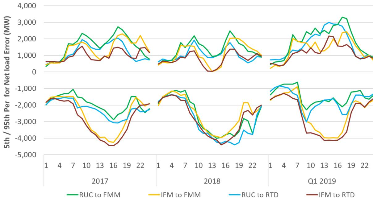
The most marked difference is observed from the IFM market to both FMM and RTD in the downward direction. This is driven largely by the inclusion of virtual bids and is observed mostly during mid-day hours when VER penetration is the highest.
