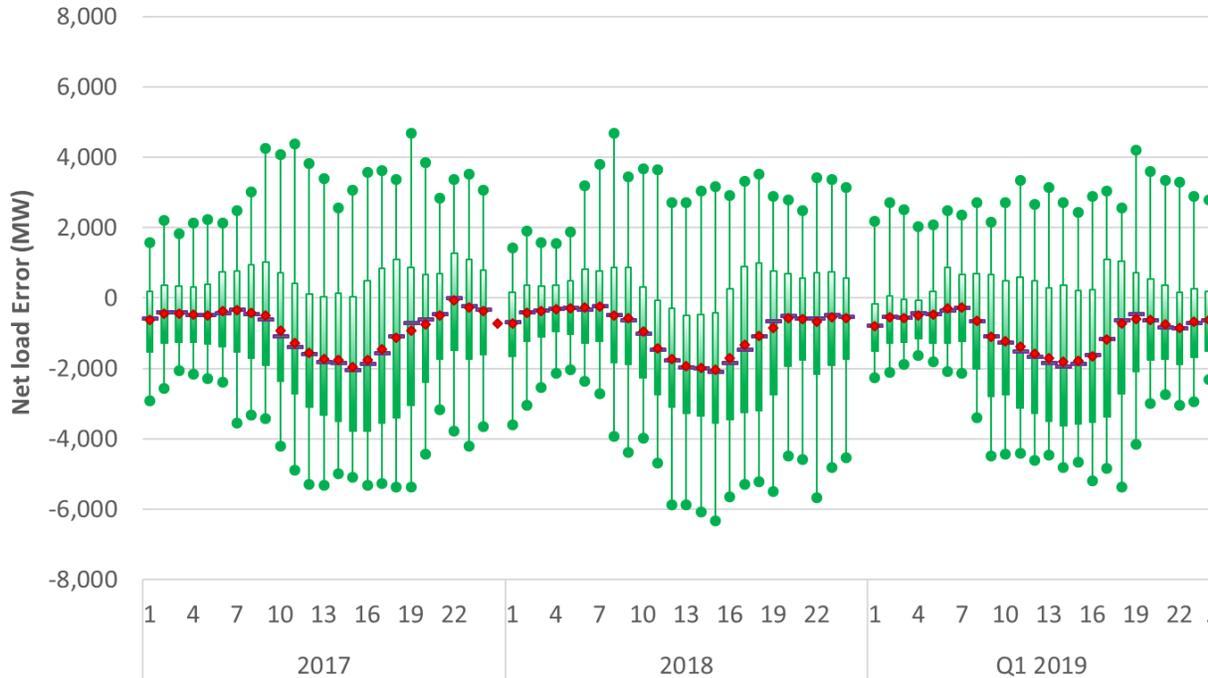
Figure 58: Hourly profile of net load differences between IFM and RTD with no load conformance
