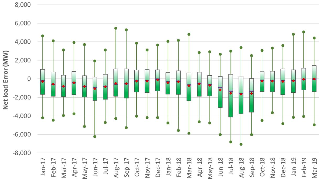
Figure 54 shows the net load errors between CAISO markets at the 5<sup>th</sup> and 95<sup>th</sup> percentile, which reflect the downward and upward net load errors between markets. These percentiles are taken as a reference to have a simpler comparison among the various levels of net load errors.
