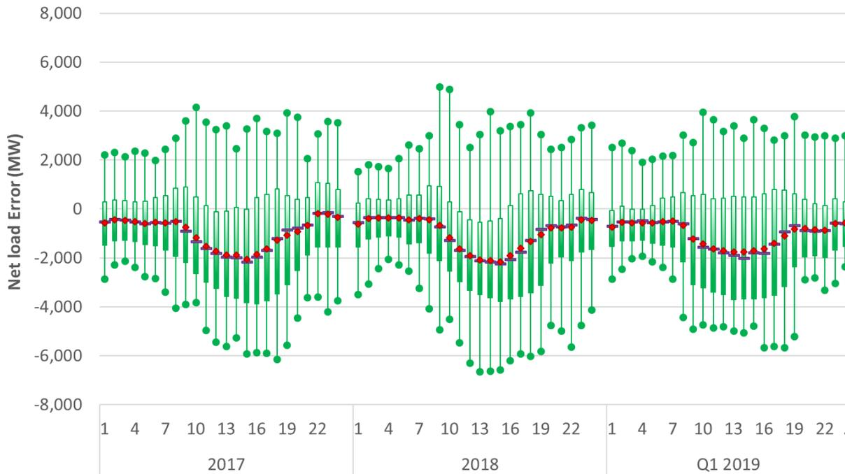
Figure 59: Hourly profile of net load differences between RUC and FMM with operator adjustments
