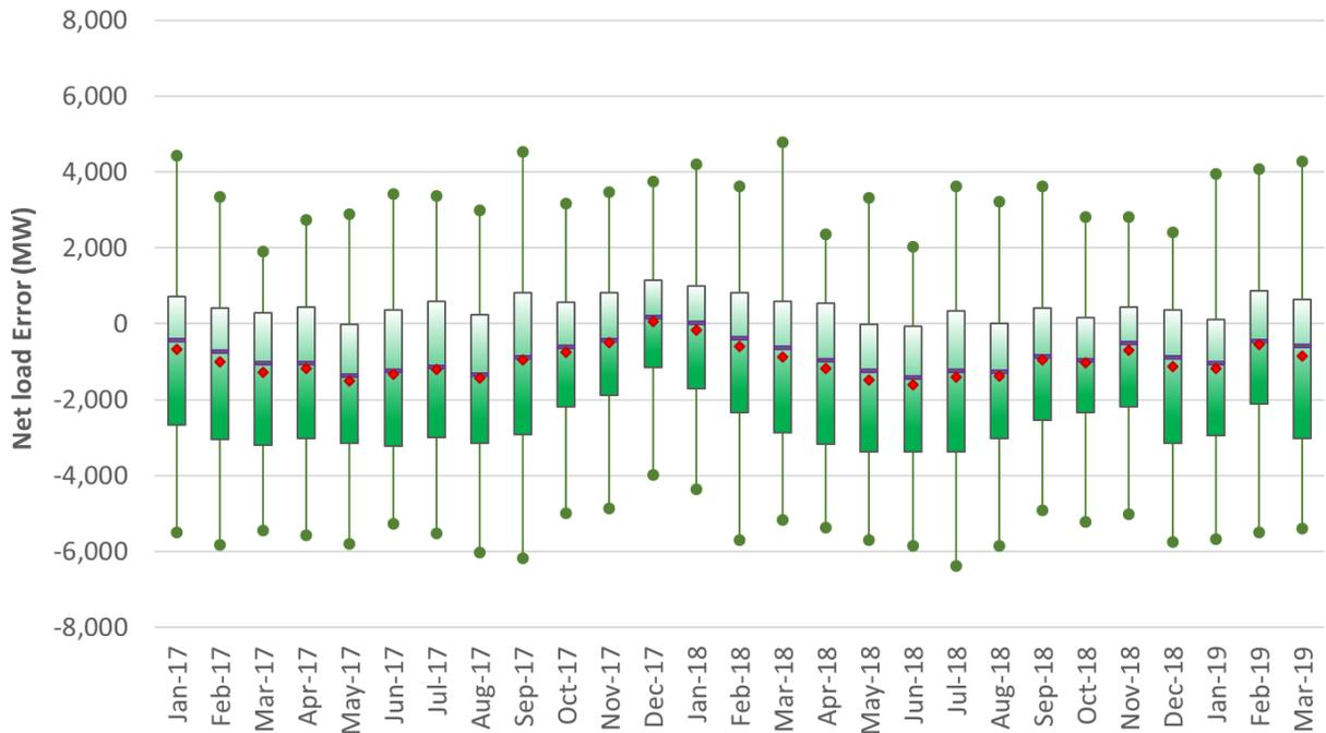
Figure 52: Monthly profile of net load differences between RUC and FMM
