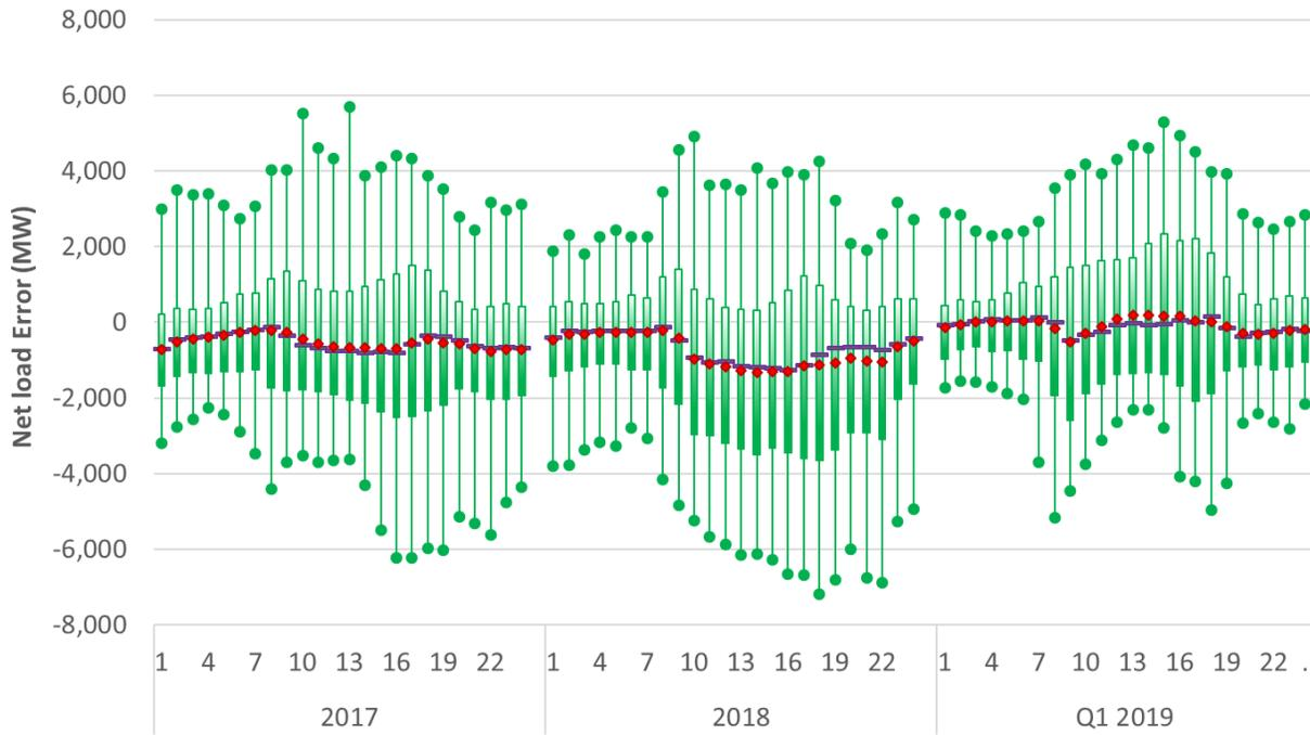
Figure 50: Monthly profile of net load differences between IFM and FMM
