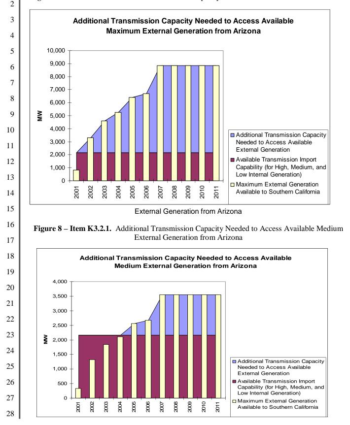
Figure 7 – Item K3.1.1. Additional Transmission Capacity Needed to Access Available Maximum
