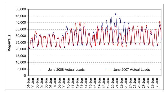
Figure 2.1 California ISO System-wide Actual Loads: June 2008 vs. June 2007
