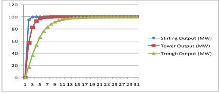
Figure 2: Response to Step Increase in Irradiance by Solar Thermal Technology v, Time in Minutes
