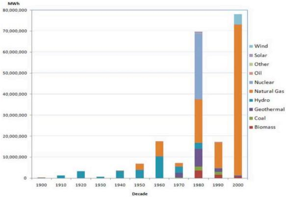
Figure 2: California In-State Electric Generation in 2009 by Generator Vintage and Fuel Type (2009 Data in MWH)<sup>35</sup>
