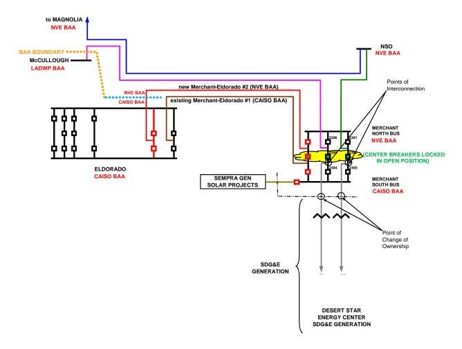
The configuration in Figure 1 will result in, south bus of Merchant Switchyard, and the Merchant-El Dorado #1 circuit being included within the CAISO BAA. The tie breakers in the 230 kV Merchant Switchyard will remain locked in open position and isolated during this interim phase and will serve as the demarcation boundary between the NVE BAA (North Bus and its associated connections) and CAISO BAA (South Bus and its associated connections).
