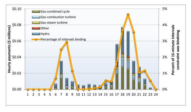
Most payments for ramping capacity occurred during the evening peak hours. Figure 1.9 shows the hourly flexible ramping payment by technology type during the first quarter. As shown in the figure, the highest payment periods were in hours ending 7 and between 17 and 21. Natural gas-fired capacity
