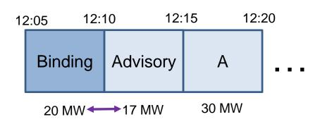
Forecasted movement = 17 MW - 20 MW = -3 MW (downward)
