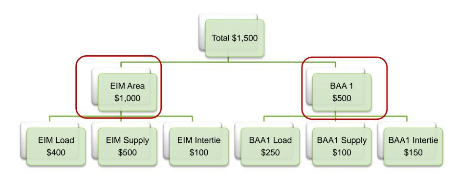
Total \$ are allocated to EIM Area and BAAs based on the constraints a resource resolve. 100 MW x \$10 for EIM area; 100 MW x \$5 for BAA 1 (see previous example)
