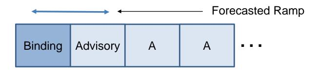
The MW difference between the first advisory interval and the binding interval in the same market run.
