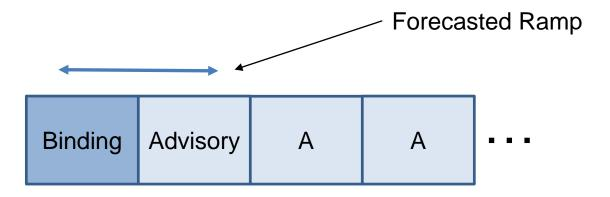
The MW difference between the first advisory interval and the binding interval in the same market run.
