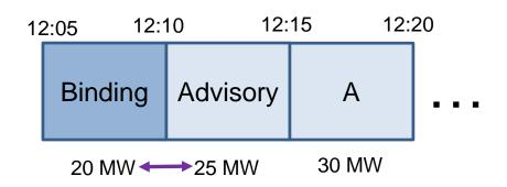
Forecasted movement = 25 MW - 20 MW = 5 MW (upward)
