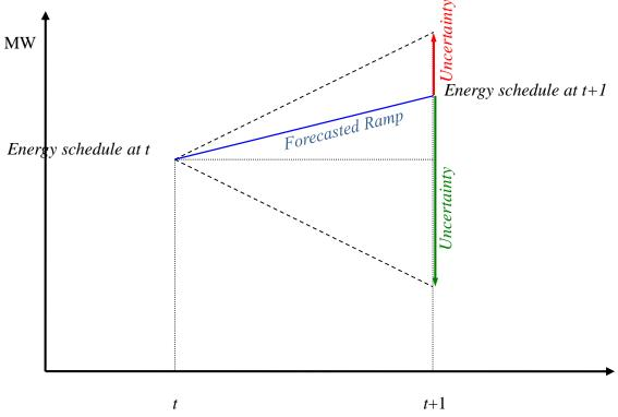
Based on historical information, the ISO determines additional upward or downward capacity that may be needed. This amount makes up the "uncertainty requirement."
