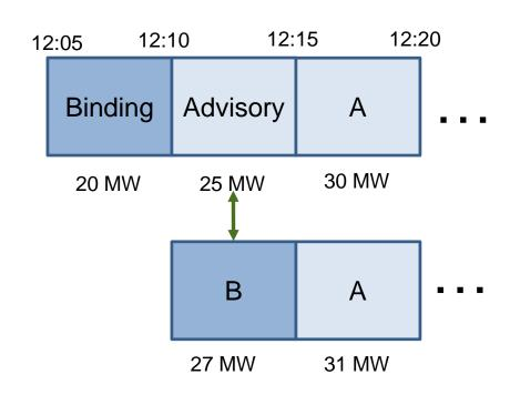
Uncertainty movement = 27 MW - 25 MW = 2 MW (upward)
