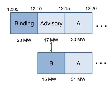
Uncertainty movement = 15 MW - 17 MW = -2 MW (downward)
