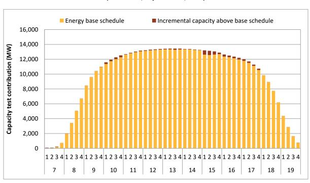
Figure 2.10 Solar resources included in CAISO's capacity test (hours 8-19, September 6, 2022)
