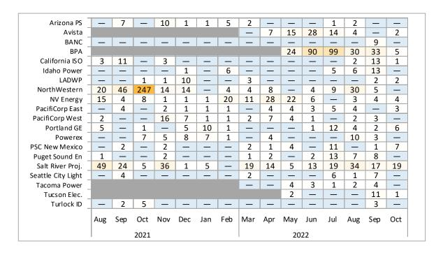
Figure 5.4 Average shortfall of upward flexibility test failures (MW)
