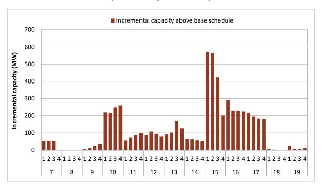
Figure 2.11 Incremental capacity from solar resources in CAISO's capacity test (hours 8-19, September 6, 2022)
