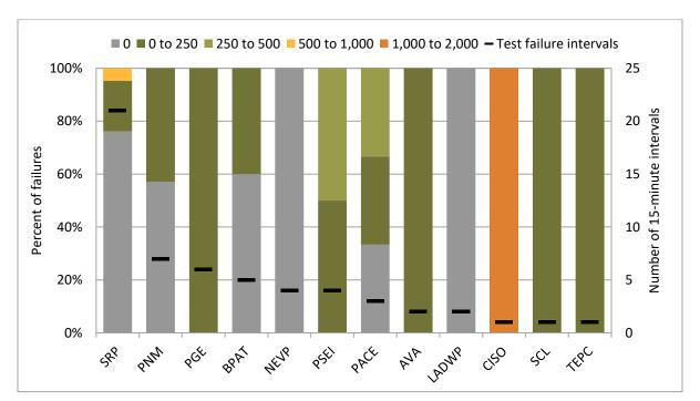
Figure 6.2 Upward capacity/flexibility test failure intervals by dynamic import limit (October 2022)
