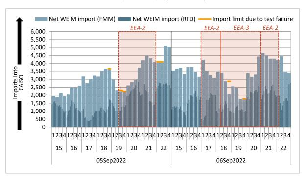
Figure 2.16 CAISO WEIM transfers and any import limit following resource sufficiency evaluation failure (peak hours, September 5-6)
