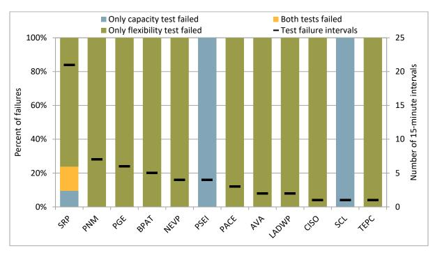
Figure 5.9 Upward capacity/flexibility test failure intervals by concurrence (October 2022)
