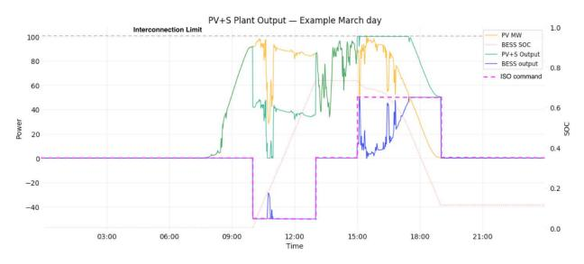
In this example, the PV has a lower bid price and therefore has the priority to generate. The on-site controller will monitor the LGIA constraint at the project substation and discharge on a second-by-second basis to fill the Interconnection Limit since it has cleared in the market. The
