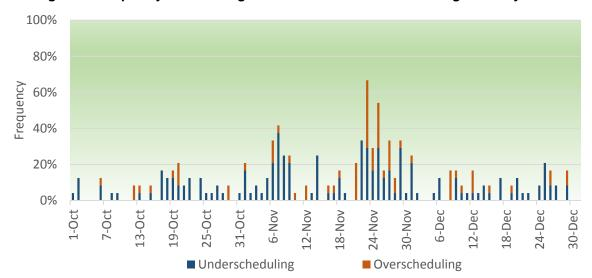
Figure 4: Frequency of balancing test failures in the APS balancing authority area.
