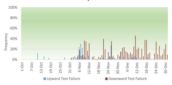
Figure 5: Frequency of flexible ramping sufficiency test failures in the APS balancing authority area.
