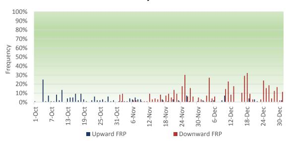
Figure 6: Frequency of flexible ramp constraint infeasibilities in the APS balancing authority area.
