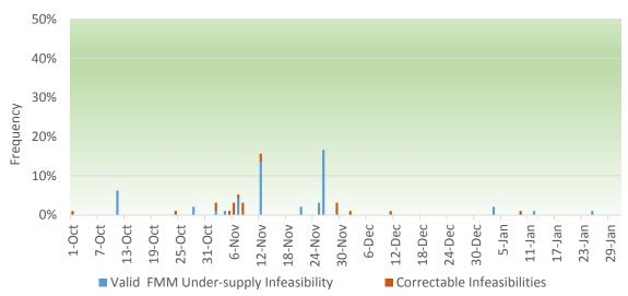
Figure 2: Frequency of FMM under-supply power balance infeasibilities in the APS balancing authority area.
