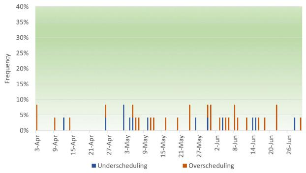
Figure 81: Frequency of Balancing Test Failures for the NV Energy BAA
