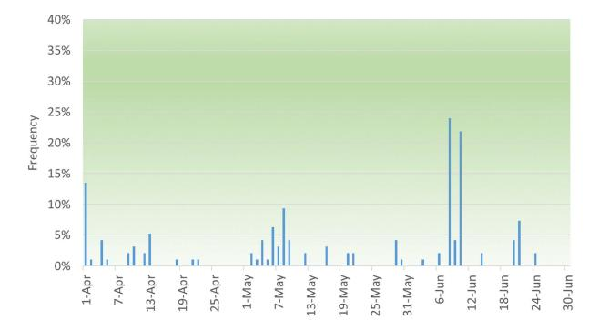
Figure 94: Frequency of Flexible Ramping Sufficiency Test Failures in the APS BAA
